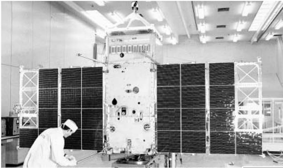
TD-1 in the integration hall at ESTEC, July 1971. The attitude control system held this side square on to the Sun.
