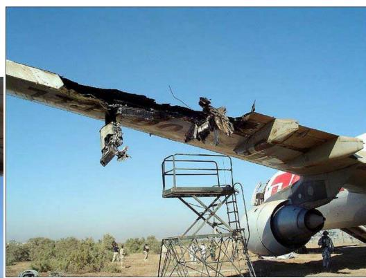
MANPADS damage on the Airbus A300
