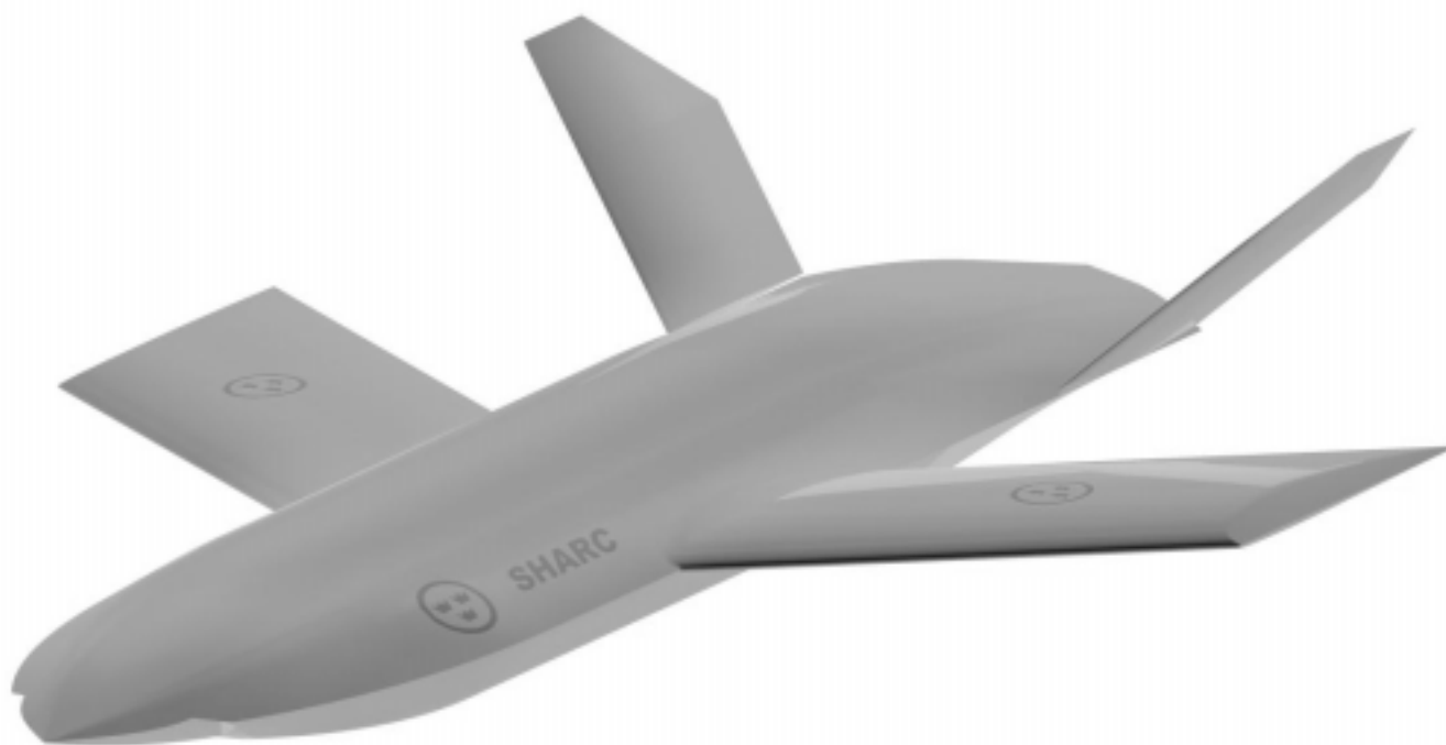
SHARC (Swedish Highly Advanced Research Configuration) Längd 10 m, spännvidd 8 m, startvikt 5 ton
