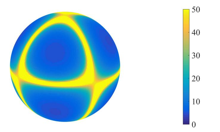
The radial distance error as a function of incidence directions. Given are: the number of listening aircraft, their nominal positions, and errors in own position and time.
