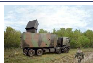
Fig. 1b: ARABEL X band MFR radar in land version (SAMP/T)
