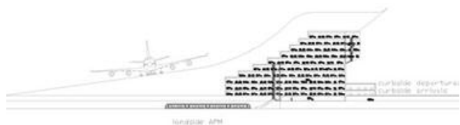
Figure 3. Space beneath the banked runway could be used for parking. (NLR)
