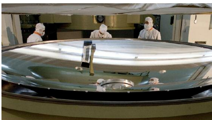
Figure 1 – Herschel Space Telescope primary mirror integrated (left) and the constituent SiC petals, the larger ever build with the selected manufacturing process. © Astrium/Boostec
