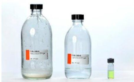
Figure 3 : Final Fischer-Tropsch products derived from solar synthetic gas. Left: Heavy product (waxes). middle: condensate from light product stream ( \text{H}_2\text{O} and hydrocarbons). Right: the world’s first solar kerosene.
