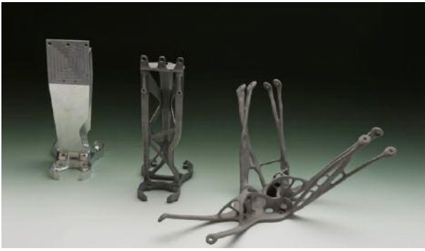
Figure 2 – Left, Evolving designs: using topology optimisation software combined with 3D printing, manufactured items can be radically different from conventional designs, often widely organic in appearance and moving towards the “bionic” design. Right, AM for planetary colonisation as demonstrated on a recent ESA study, where a 1.5 tonnes lunar regolith moon base segment has been successfully additive manufactured (artist impression). © ESA/Foster Partners
