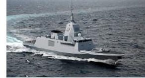
Fig. 4b: Sea Fire S band radar as integrated on a large Frigate.
