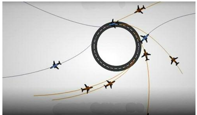
Figure 7. Traffic could approach and leave an endless runway from any direction. (NLR)
