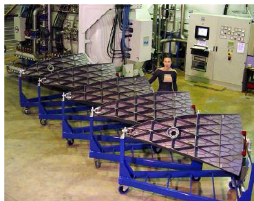
Figure 1 – Herschel Space Telescope primary mirror integrated (left) and the constituent SiC petals, the larger ever build with the selected manufacturing process. © Astrium/Boostec
