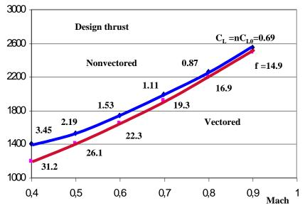
Fig. 15.9 Turning radius vs Mach number
