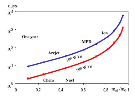
Fig. 23.8 Operating time with optimum payload
