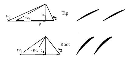
Fig. 13.9 Blade shapes at tip and at root.
