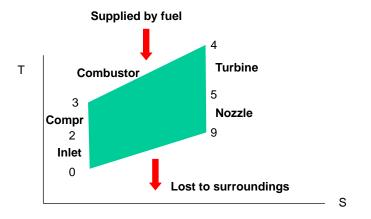
Fig. 8.8 The jet engine follows the Brayton cycle
