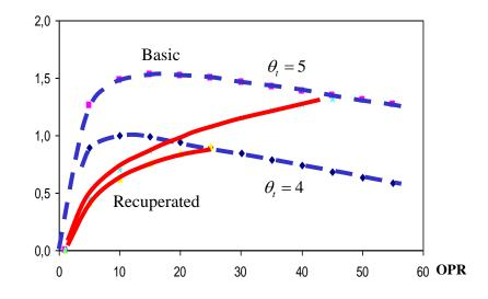
Fig. 14.4 Recuperated power with pressure
