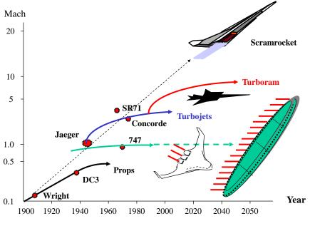
Fig. 24.1 The future of airbreathing propulsion
