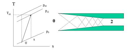
Fig. 18.3 Pressure loss in inlets
