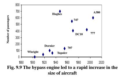
In the 1920's it was realized that the technology at the time did not permit the building of very large aircraft starting from the ground. This was the reason for the flying boats of which the Dornier "Do X" and the Hughes "Spruce Goose" were the largest.
