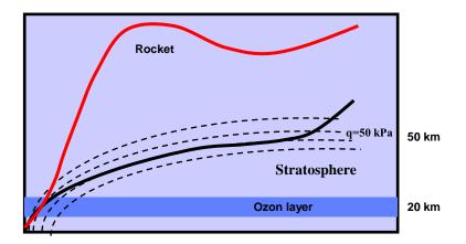
Fig. 22.5 Spaceplane and rocket trajectories
