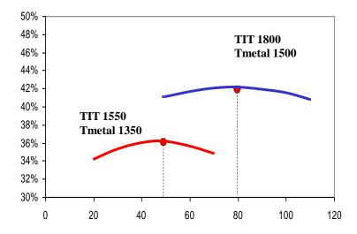
Fig. 12.12 There is an Overall Pressure Ratio (OPR) that maximizes the efficiency
