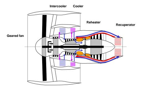
Fig. 14.1 Ducted propfan Intercooler-Reheater-Recuperator
