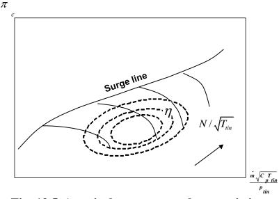
Fig. 13.5 A typical compressor characteristics
