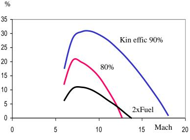
Fig. 19.7 The efficiency of a Scramjet
