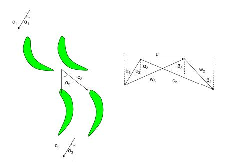
Fig. 13.17 Turbine cascade with velocity triangles
