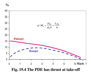
The main deficiency of the ramjet is immediately obvious, namely that the thrust vanishes at low speed. It is therefore impossible to use it from take-off. It needs another engine to give it the speed
