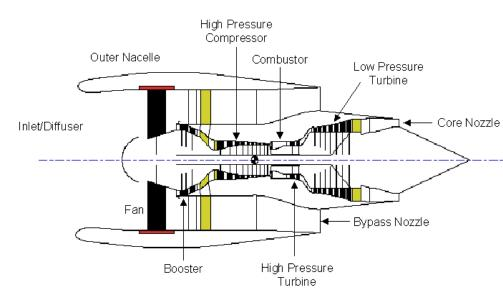
Fig. 9.7 The components of the bypass engine
