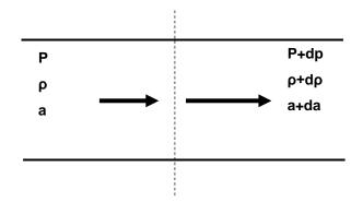
Fig. 7.9 Shock moving through a tube
