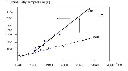
Fig. 12.10 The increase of the Turbine Entry Temperature
