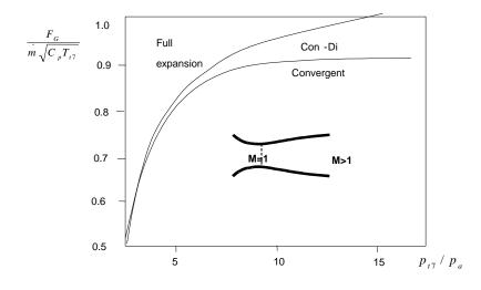
Fig. 16.8 Gross thrust from nozzles
