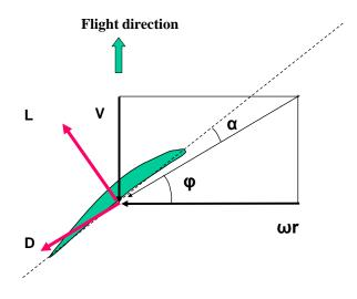
Fig. 7.6 Forces on a propeller
