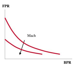
Fig. 9.6 The variation of fan pressure ratio with bypass ratio and Mach number
