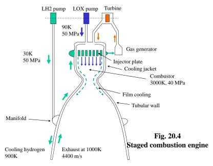
From the outside, a liquid-propellant engine often looks like a maze of plumbing, which connects the tanks to the pumps, carries the coolant flow to and from the cooling jackets, and conveys the pumped fluids to the injector. In addition, engines are generally
