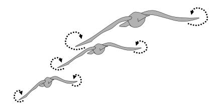
Fig. 4.2 The wing tip vortex creates an upwash
