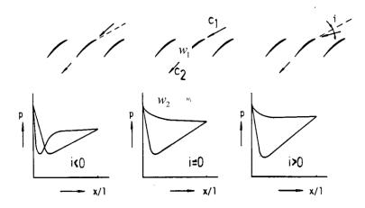
Fig. 13.7 Pressure variation at different incidence angles
