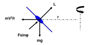
Fig. 15.7 Forces on a turning aircraft
