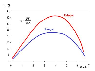
Fig. 19.3 The PDE is more efficient than the ramjet
