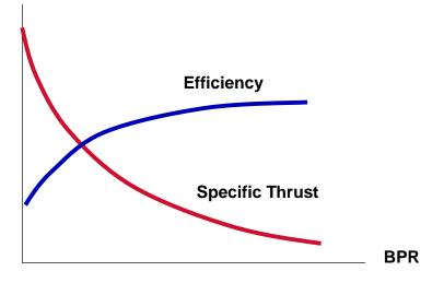
Fig. 9.4 The behaviour of specific thrust and efficiency with bypass ratio
