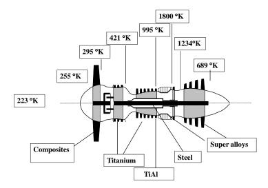
Fig. 13.1 The turbomachinery of the new civil engine
