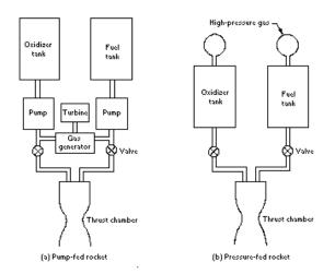
Fig. 20.2 Pump-fed and pressure-fed liquid rocket engines
