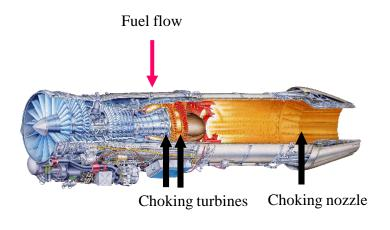
Fig. 17.3 Parameters influencing off-design behavior
