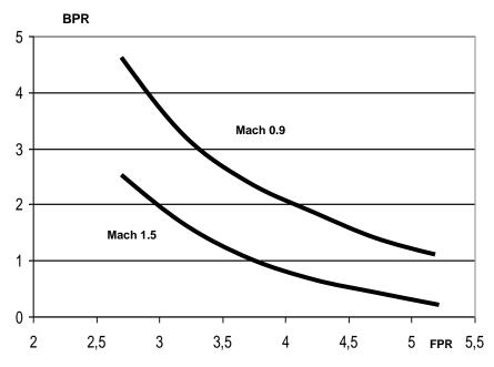
Fig. 16.12 The bypass ratio decreases with fan pressure ratio
