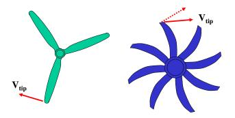
Fig. 7.11 The blades are swept to increase the speed of propellers
