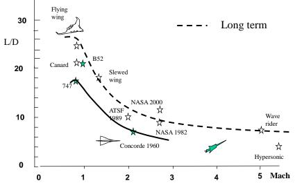
Fig. 11.7 The L/D falls rapidly at higher Mach numbers
