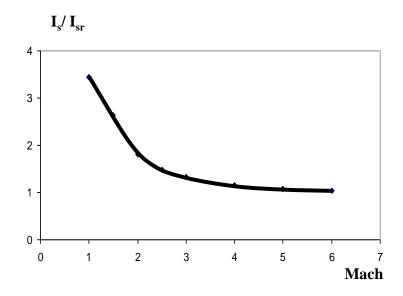
Fig. 21.8 The specific impulse of a LACE compared to a rocket
