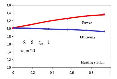
Fig. 14.6 Power and efficiency with reheating
