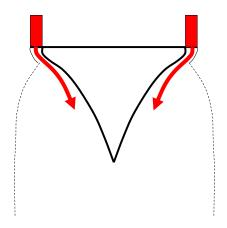
Fig. 20.5 Aerospike nozzle
