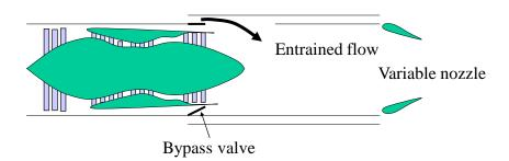
Fig. 17.8 Choked bypass ejector nozzle engine
