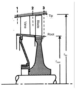
Fig. 13.15 Turbine stage
