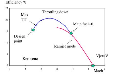
Fig. 18.4 Turboramjet efficiency versus Mach number
