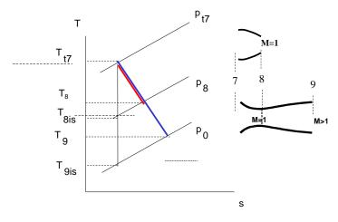
Fig. 16.7 Expansion in a convergent-divergent and in a convergent nozzle
