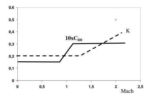
Fig. 15.6 Coefficients to calculate total drag
