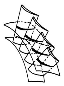
Fig. 13.3 Blade stream surfaces
