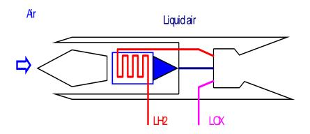
Fig. 21.7 Liquid Air Combustion Engine (LACE)
