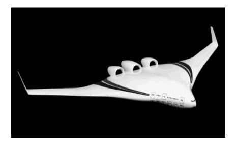
Fig. 11.10 The blended body aircraft
