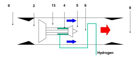
Fig. 21.3 In the Turboramexpander, the heated fuel is used to drive the turbine
