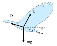
Fig. 4.3 Forces on the bird and the gliding angle
