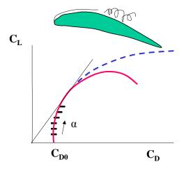
Fig. 6.4 The maximum L/D is at the tangent to the drag polar
