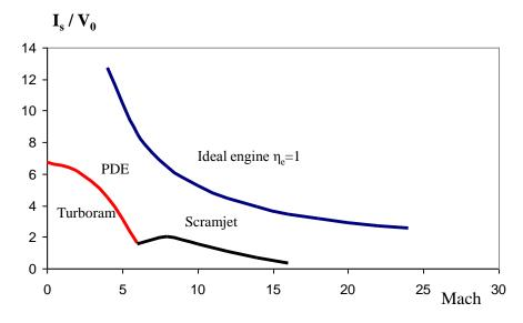
Fig. 24.2 Limits to airbreathing propulsion
