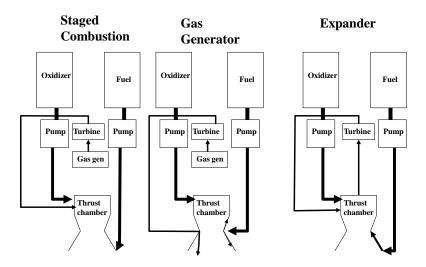
Fig. 20.3 Pump-fed liquid rocket engine cycles
