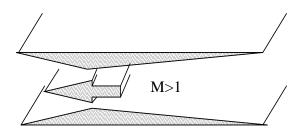
Fig. 19.6 The supersonic ramjet (Scramjet)
