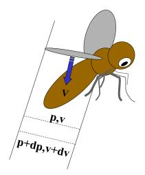
Fig. 3.4 The reaction force is balanced by a pressure force below the wings.
