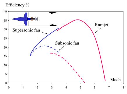
Fig. 18.5 Increased efficiency with a supersonic fan
