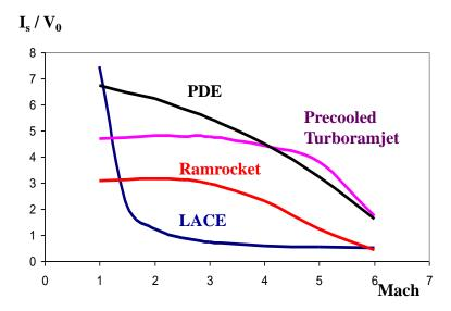
Fig. 21.9 Specific impulse of engines for speeds below Mach 6
