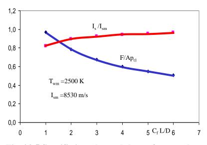
Fig. 23.5 Specific impulse and thrust for a nuclear engine
