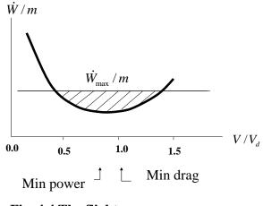
Fig. 4.4 The flight power curve
