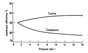
Fig. 12.4 Isentropic efficiency for compressors and turbines at constant polytropic efficiency 0.85
