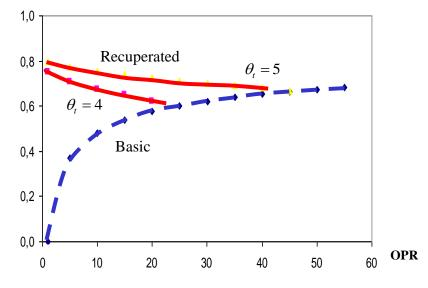
Fig. 14.3 Variation of recuperated thermal efficiency with pressure
