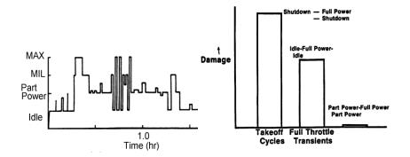
Fig. 17.1 The operating cycle of a military engine
