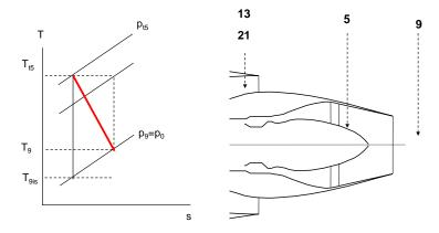
Fig. 12.8 Expansion with losses in the nozzle
