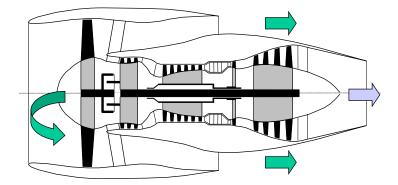
Fig. 9.1 In the bypass engine part of the power is used to drive a fan
