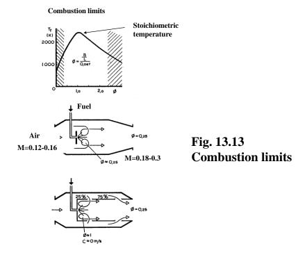
Fuel without oxygen will not burn, neither will oxygen without fuel. The two extremes of mixture ratio are termed the lean- and rich limit mixtures, the former when oxygen is in excess and the latter when fuel is in excess. The magnitude of these limits depends somewhat on the composition of the fuel but for ordinary hydrocarbons they are in the range A/F=5-25 that is the stoichiometric air to fuel ratio is somewhere in between.
