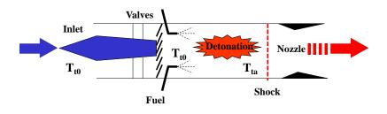
Fig. 19.2 The principle of a Pulse Detonation Engine
