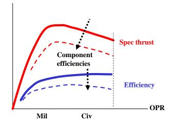
Fig. 9.5 The behaviour of specific thrust and efficiency with pressure ratio
