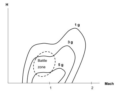
Fig. 15.8 Sustained turn flight envelops for different load factors
