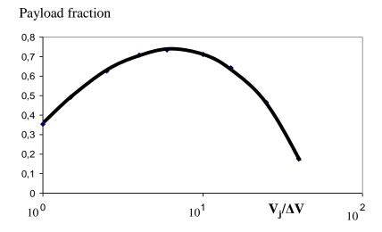
Fig. 23.6 Earth-Mars mission payload fraction
