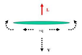
Fig. 3.5 Air leaking around a wing moving down
