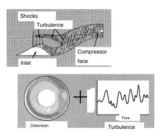
**Fig. 16.5 Distorsion patterns in inlets**
