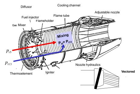
Fig. 16.6 The afterburner and nozzle distinguishes a military engine
