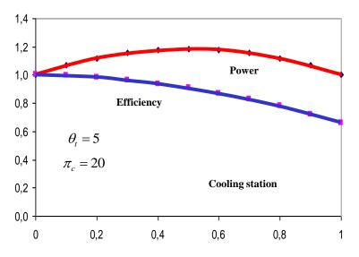
Fig. 14.5 Power and efficiency with intercooling
