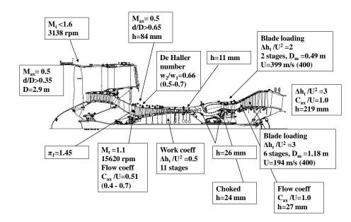
Figure 13.18 The Advanced Civil Engine 2020
