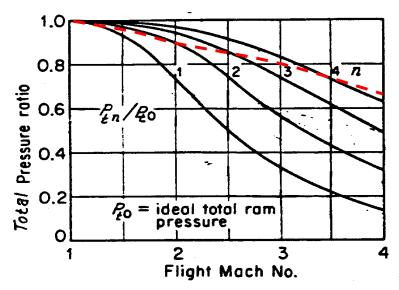
Fig. 16.4 The pressure loss in supersonic inlets
