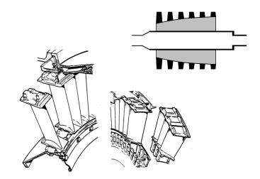
Fig. 13.2 Axial flow compressor blades and vanes
