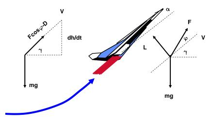
Fig. 15.4 Forces on a climbing aircraft
