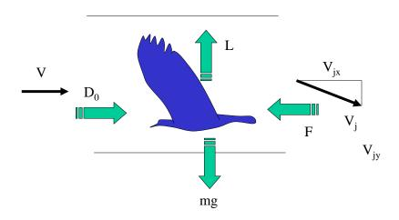
Fig. 4.1 Birds make use of the living force of a large air flow
