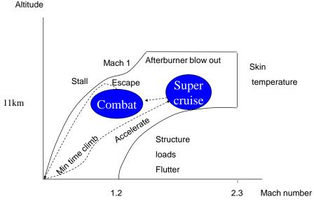
Fig. 15.3 The operating envelope for a fighter aircraft
