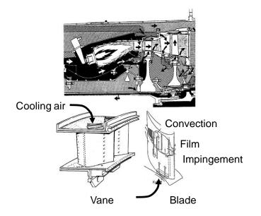
Fig. 13.14 Turbine with cooling flows
