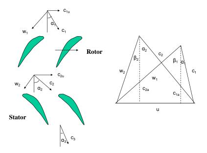
Fig. 13.4 Cascade flow and velocity triangles
