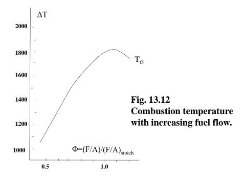
Since the gas temperature determines the engine thrust, the combustion chamber must be capable of maintaining stable and efficient combustion over a wide range of engine operating conditions. Experiments have shown that there are certain limits to
