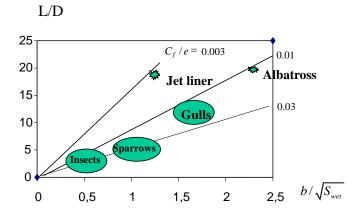
Fig. 5.5 The Lift-to-Drag ratio of birds
