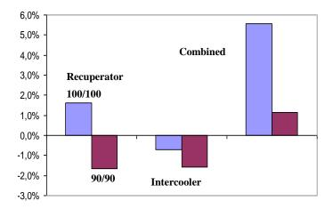
Fig. 14.7 Effect of heat exchangers on engine efficiency
