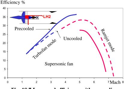
Fig. 18.7 Increased efficiency with precooling
