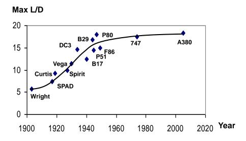
Fig. 11.8 Stagnating Lift/Drag ratio
