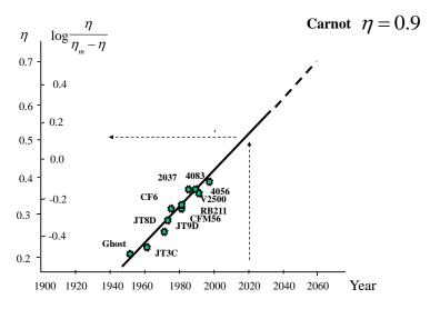
Fig. 11.6 A logistic prediction of the engine efficiency
