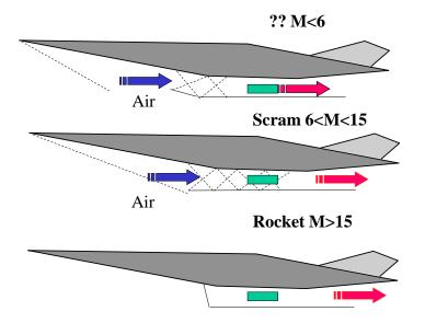
Fig. 21.1 Spaceplane propulsion phases
