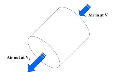
Fig. 2.4 The airbreathing engine.
