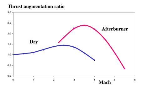
Fig. 21.5 The ratio between the ramrocket thrust and the rocket thrust.
