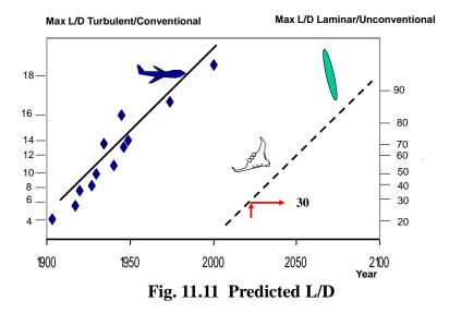
Now assume that we want to design an aircraft and an engine for the 2020s. Such an aircraft would have a L/D ratio of 30 compared to 19 for the A380. This can be used to find the thrust of the engine.
