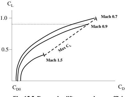
Fig. 15.5 Drag polar-lift versus drag coefficient
