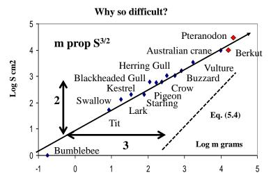
Fig. 5.2 The Law of Two Thirds shows that the weight grows faster than the area
