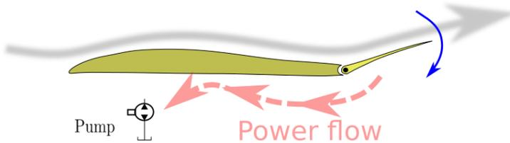
Figure 3. Power from the control surface to the pump
