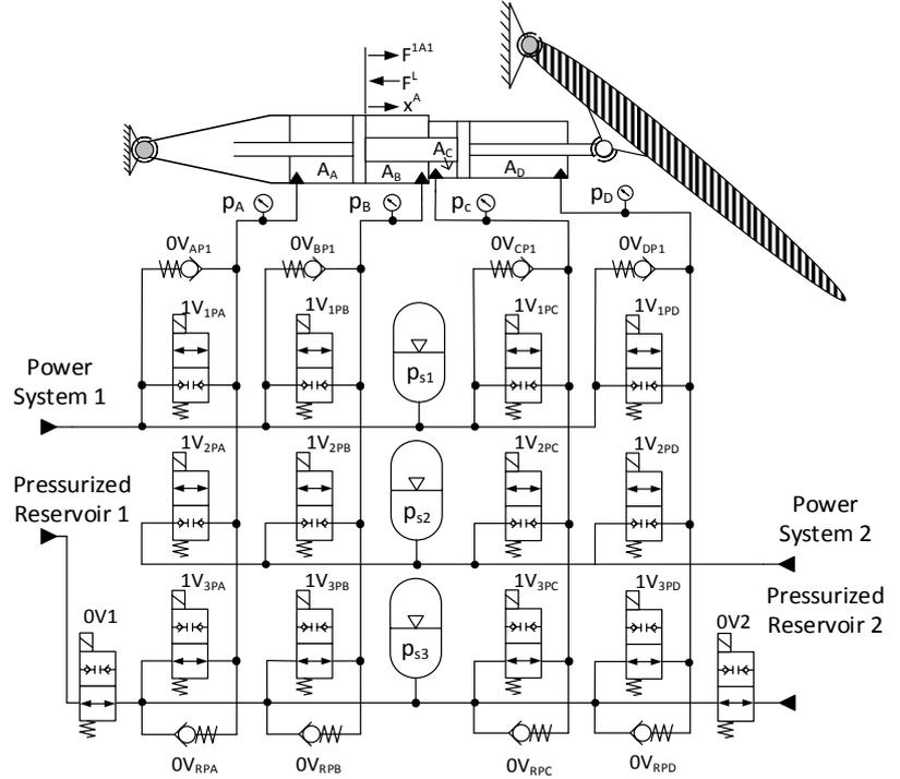
Figure 6. Digital hydraulic concept (Belan, et al., 2016)
