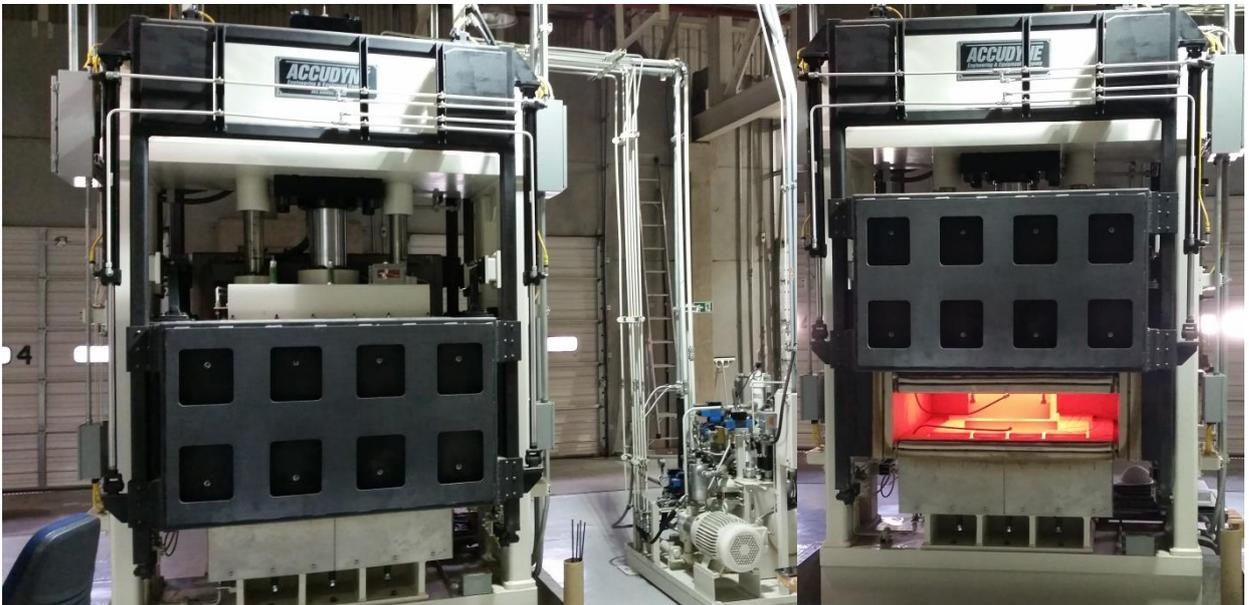
**Figure 5 –Lightweight Structures Laboratory's superplastic forming Accudyne machine.**
