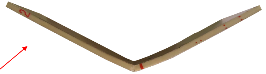
Metal-composite+Pins-metal Hexagonal pattern/spacing of 10 mm
