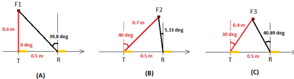
Fig. 3 – Triangulation process
