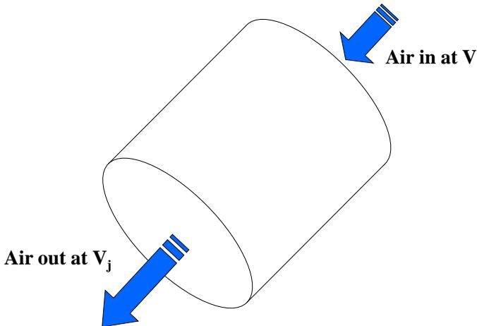
**Fig. 2.4 The airbreathing engine.**
