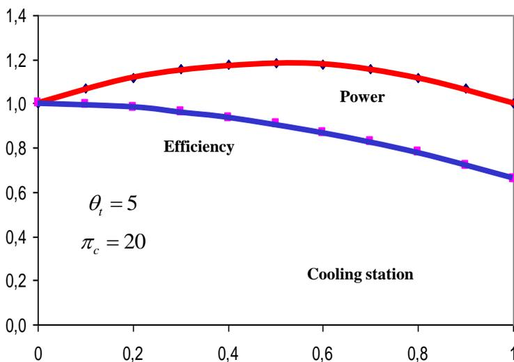
**Fig. 14.5 Power and efficiency with intercooling**
