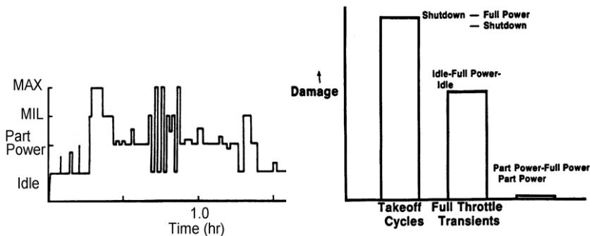
**Fig. 17.1** The operating cycle of a military engine
