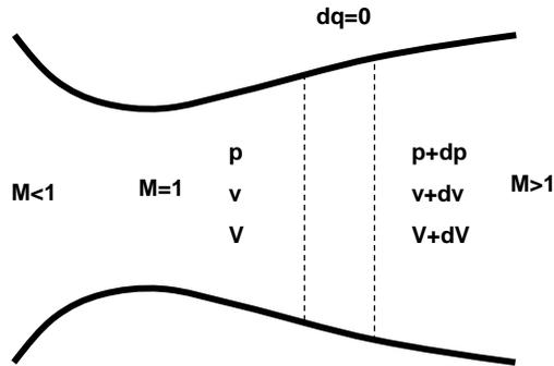
**Fig. 8.1 The Laval nozzle produces a supersonic jet**
