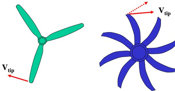
**Fig. 7.11 The blades are swept to increase the speed of propellers**
