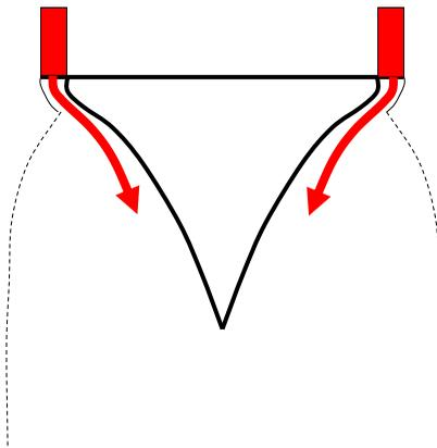
**Fig. 20.5 Aerospike nozzle**
