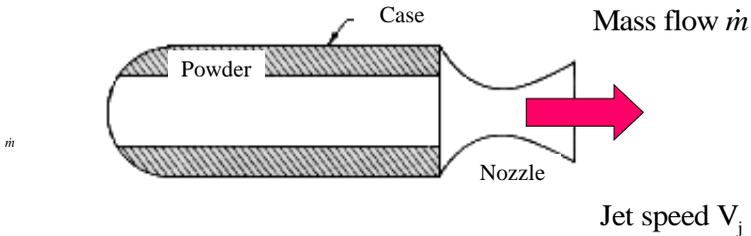
**Fig. 2.3 The solid rocket-the simplest of all reaction engines**
