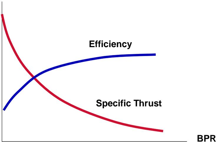
**Fig. 9.4 The behaviour of specific thrust and efficiency with bypass ratio**
