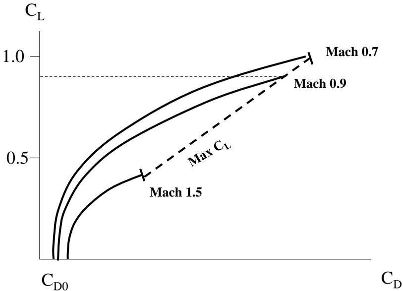
**Fig. 15.5 Drag polar-lift versus drag coefficient**
