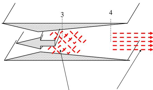
**Fuel injection shock waves and incomplete combustion are problems with the scramjet.**
