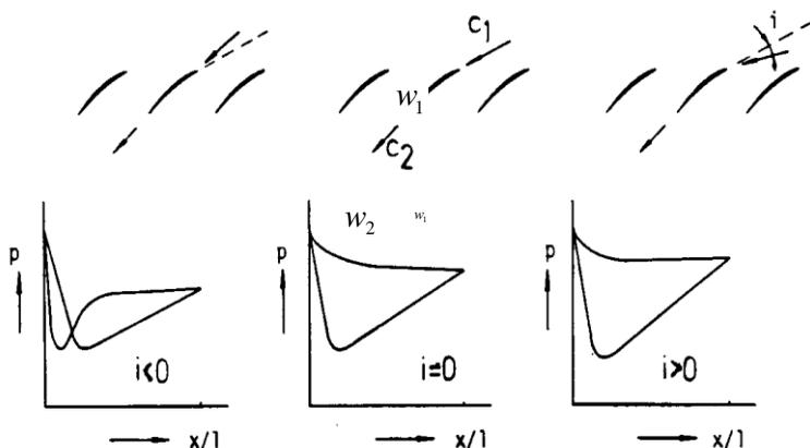
**Fig. 13.7 Pressure variation at different incidence angles**
