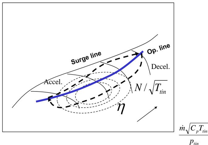
**Fig. 17.6 Acceleration and deceleration**
