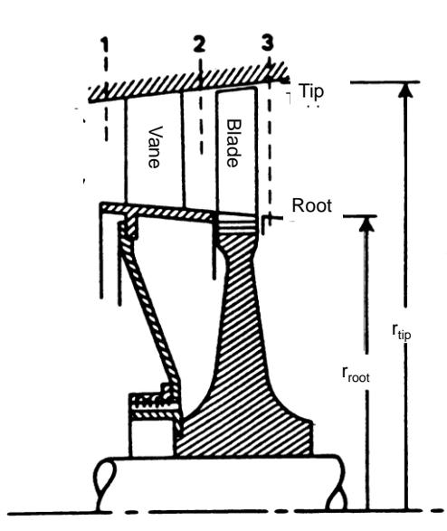
**Fig. 13.15 Turbine stage**
