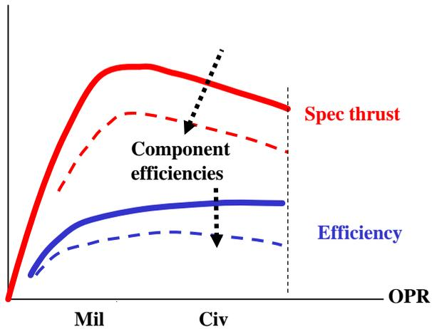
**Fig. 9.5 The behaviour of specific thrust and efficiency with pressure ratio**
