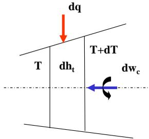
**Fig. 12.5 Control volume of the compressor**
