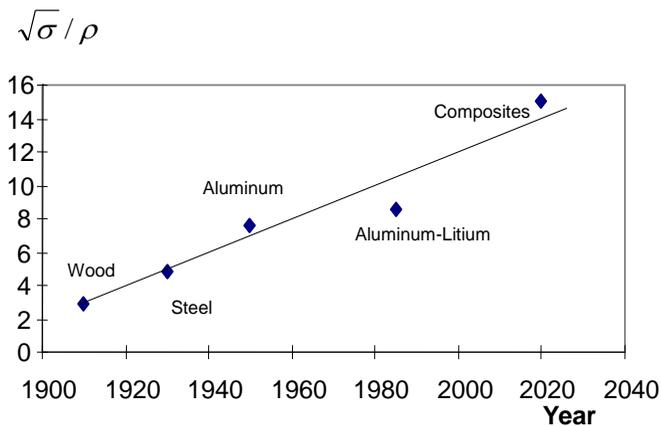
**Fig. 11.3** The growth in strength of aircraft materials
