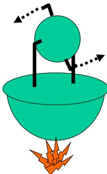
**Fig 2.2 Heron's Aeolipile-the first reaction machine?**
