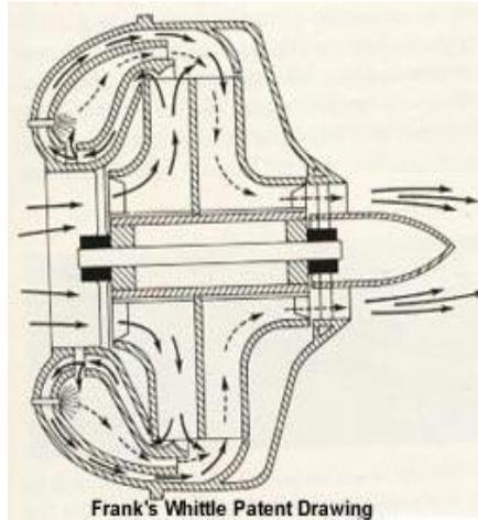
**Fig. 8.5 Frank Whittle patented the jet engine in 1930**
