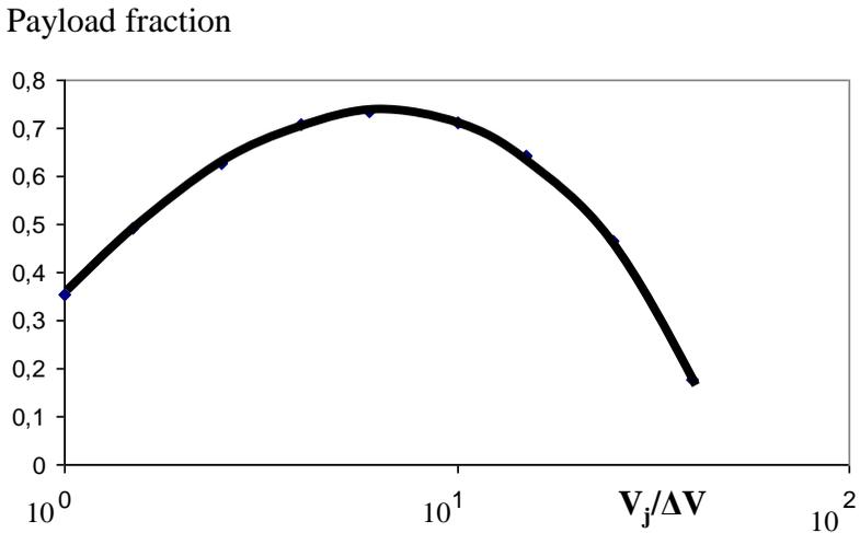
**Fig. 23.6 Earth-Mars mission payload fraction**
