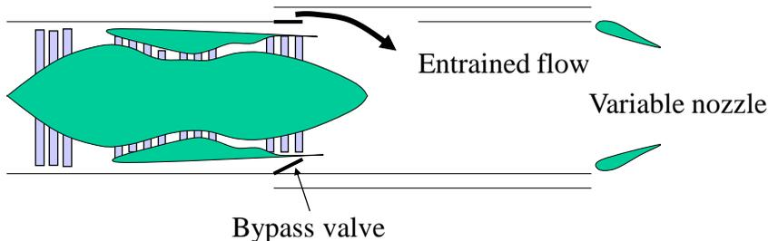
**Fig. 17.8 Choked bypass ejector nozzle engine**
