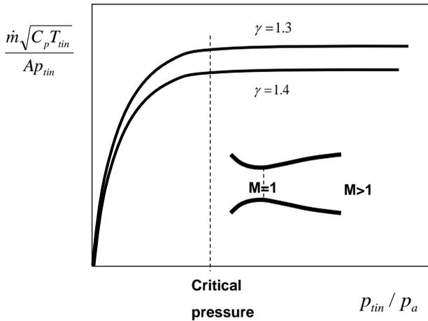
**Fig. 8.3 The variation of the mass flow with pressure in a nozzle**
