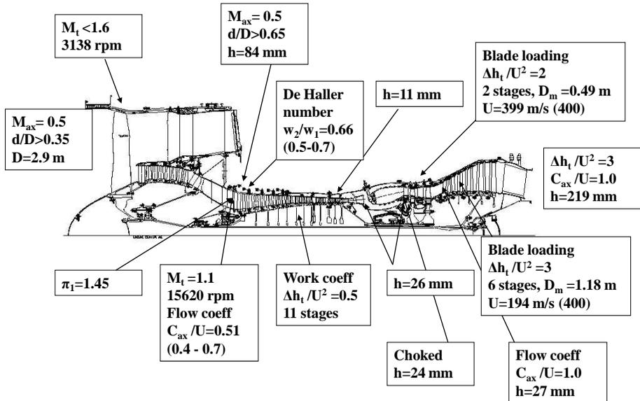
**Figure 13.18 The Advanced Civil Engine 2020**
