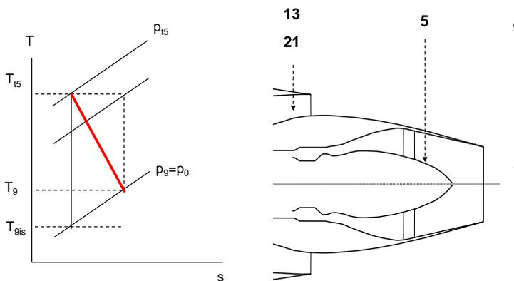
**Fig. 12.8** Expansion with losses in the nozzle
