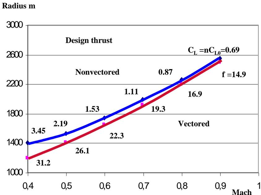
Fig. 15.9 Turning radius vs Mach number
