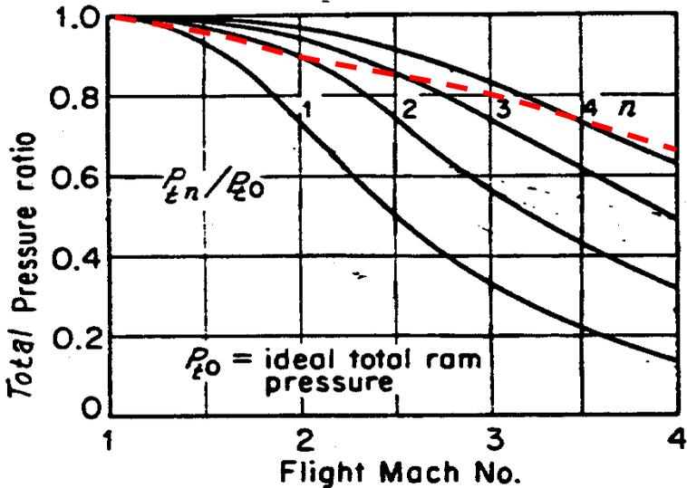
Fig. 16.4 The pressure loss in supersonic inlets
