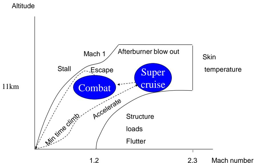
**Fig. 15.3 The operating envelope for a fighter aircraft**
