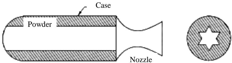
**Fig. 20.1 The solid propellant rocket**
