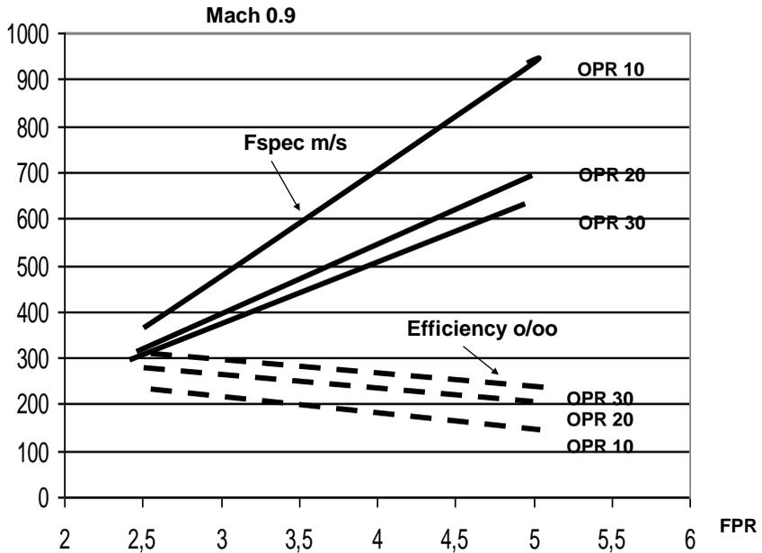
**Fig. 16.10 Specific thrust and efficiency versus OPR and FPR**
