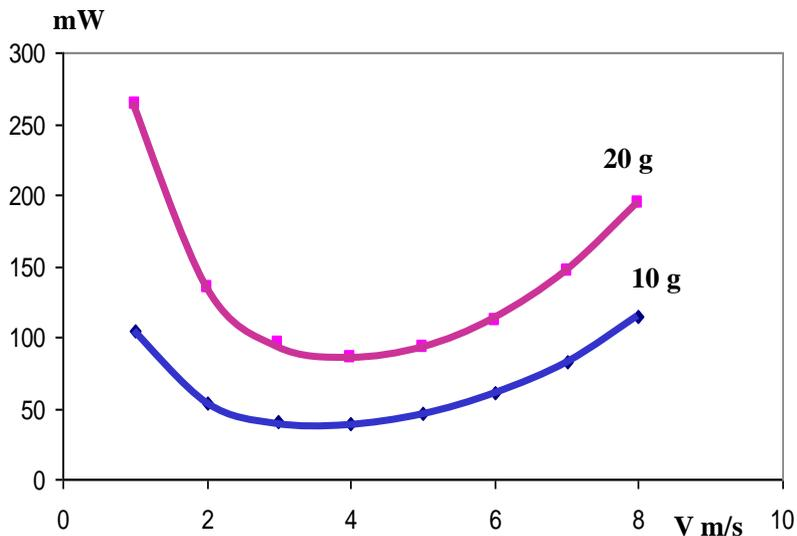
**Fig. 5.3 Micro Air Vehicle power vs speed**
