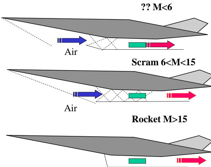
**Fig. 21.1** Spaceplane propulsion phases
