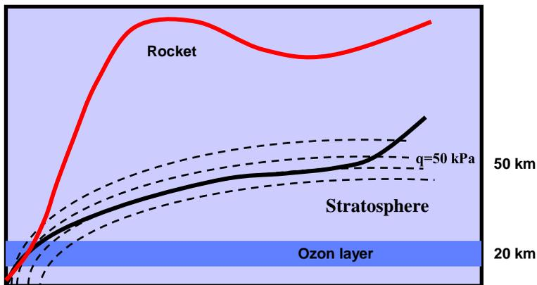
**Fig. 22.5 Spaceplane and rocket trajectories**
