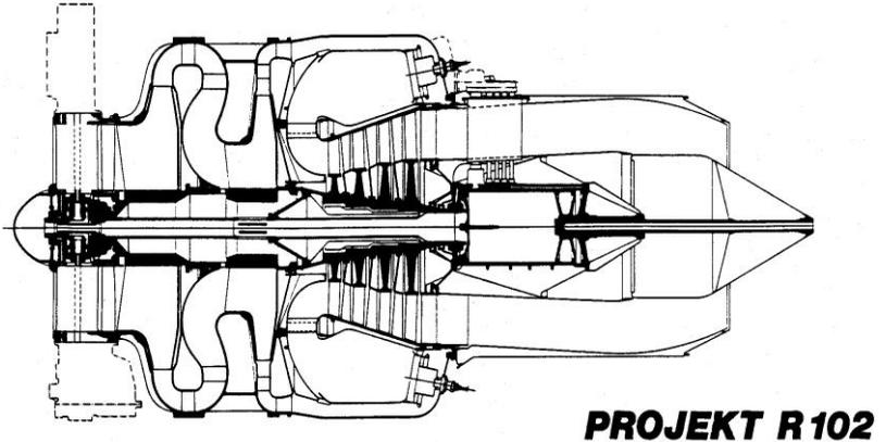
**Fig. 8.7 Volvo's first jet engine**
