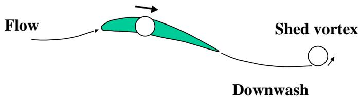
**Fig. 7.3 Prandtl detected the shed vortices from an airfoil**
