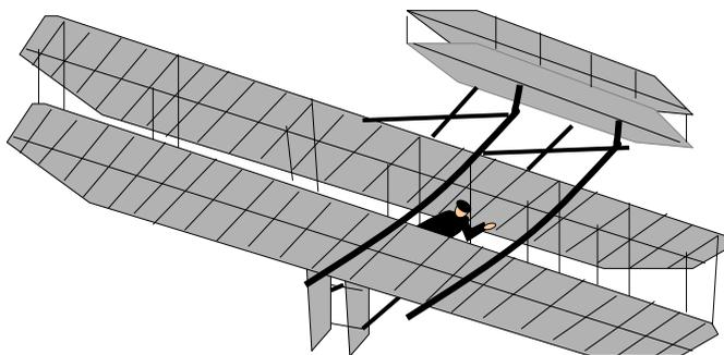
**Fig. 6.5 The Wright Flyer was the first machine to reach the power density of a bird**
