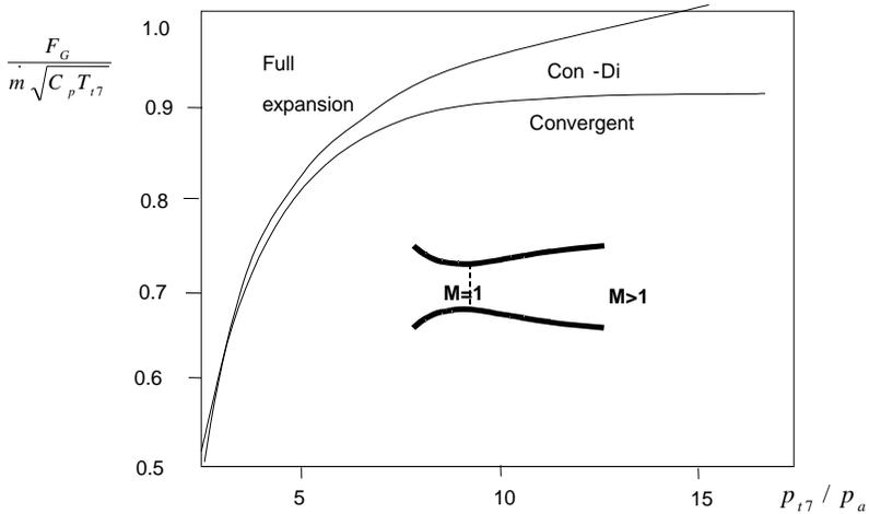
**Fig. 16.8 Gross thrust from nozzles**
