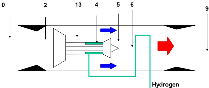
**Fig. 21.3 In the Turboramexpander, the heated fuel is used to drive the turbine**
