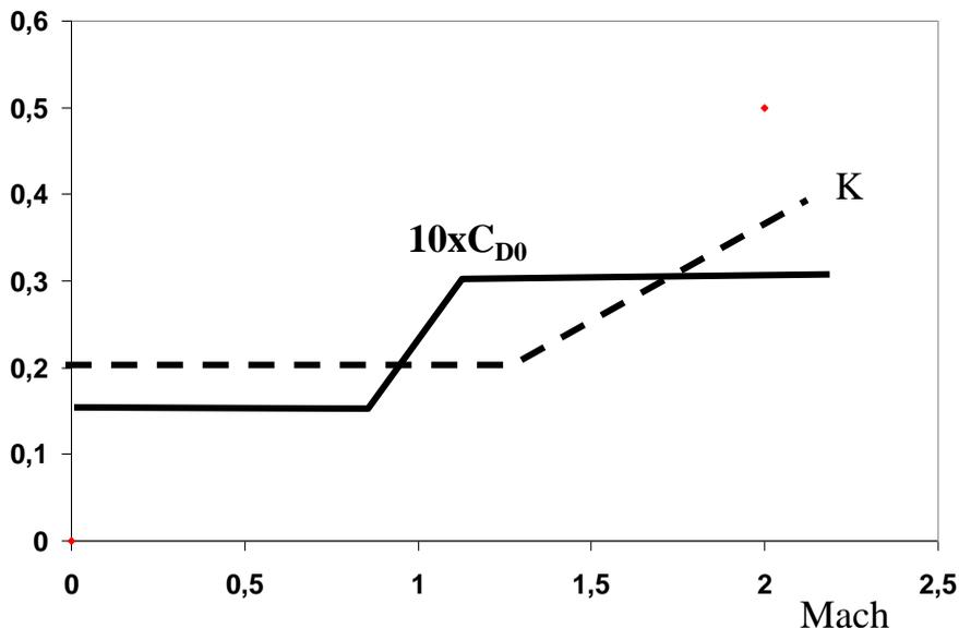
**Fig. 15.6 Coefficients to calculate total drag**
