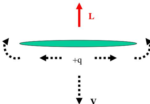
**Fig. 3.5 Air leaking around a wing moving down**
