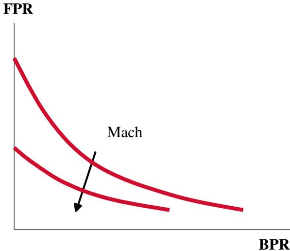
**Fig. 9.6 The variation of fan pressure ratio with bypass ratio and Mach number**
