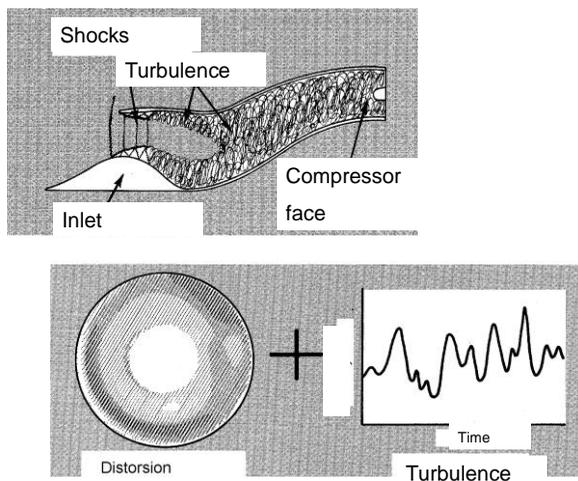
**Fig. 16.5 Distorsion patterns in inlets**
