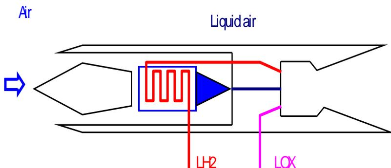
**Fig. 21.7 Liquid Air Combustion Engine (LACE)**
