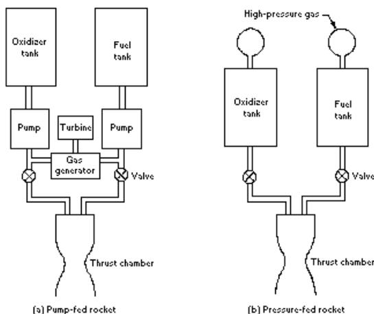
**Fig. 20.2 Pump-fed and pressure-fed liquid rocket engines**
