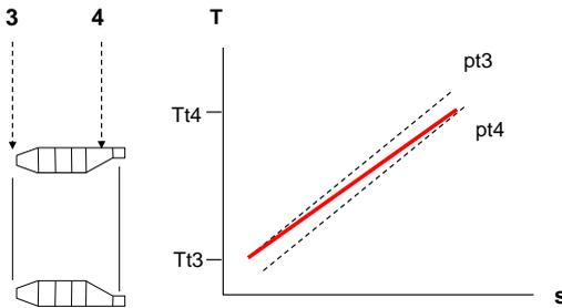
**Fig. 12.6 Combustion takes place at nearly constant pressure**
