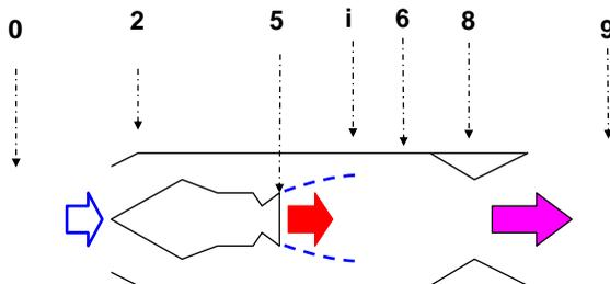
**Fig. 21.4 In the Ramrocket thrust at take-off is produced by an ejector rocket**
