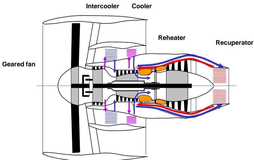
**Fig. 14.1 Ducted propfan Intercooler-Reheater-Recuperator**
