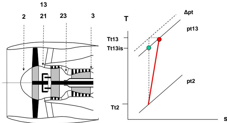
**Fig. 12.3 Heat and pressure losses in fans and compressors**
