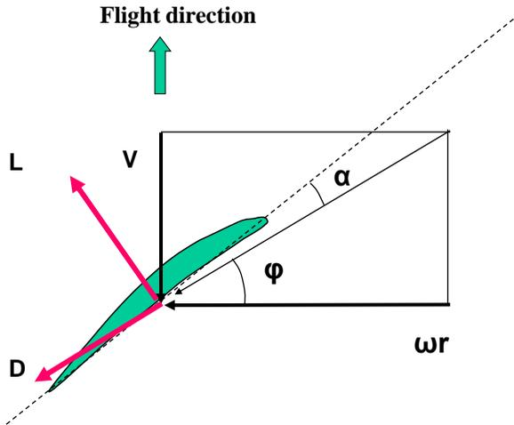
**Fig. 7.6 Forces on a propeller**
