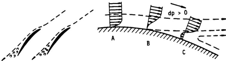
**Fig. 13.6 Separation of a flow against increased pressure**
