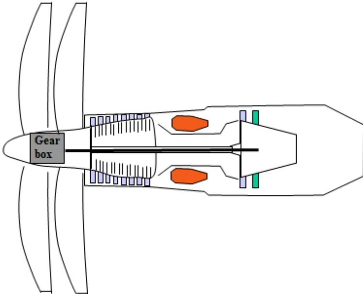
**Fig. 9.8 In the turboprop engine, the propeller is exposed to the full air flow**
