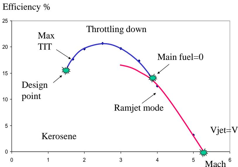
**Fig. 18.4 Turbooramjet efficiency versus Mach number**
