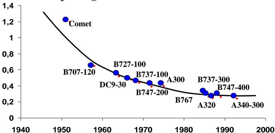
Fig. 11.1 The fuel consumption of aircraft has decreased
