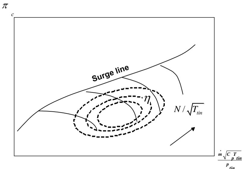
**Fig. 13.5** A typical compressor characteristics
