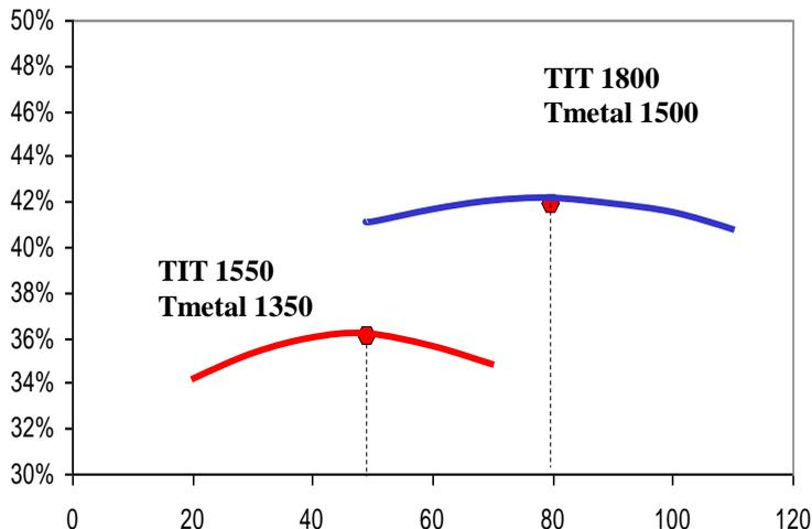
**Fig. 12.12** There is an Overall Pressure Ratio (OPR) that maximizes the efficiency
