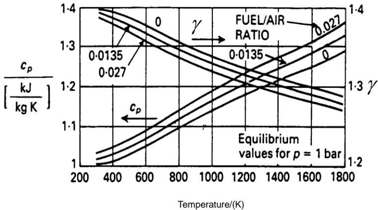
**Fig. 8.2** The specific heat and the adiabatic constant vary with temperature.
