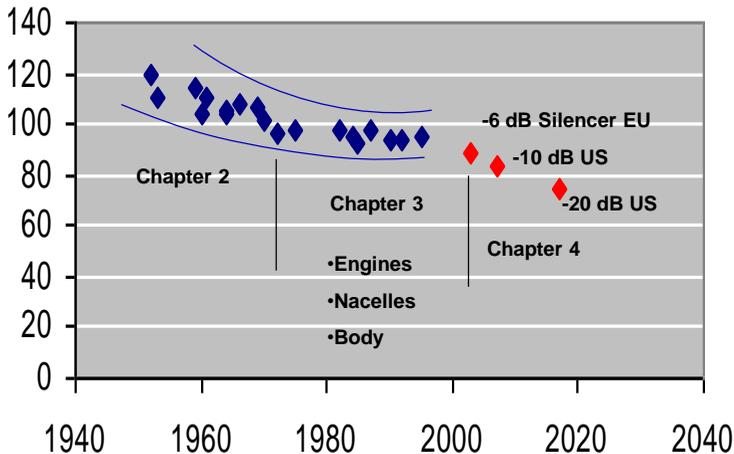
**Fig. 10.2 Noise has been substantially reduced**
