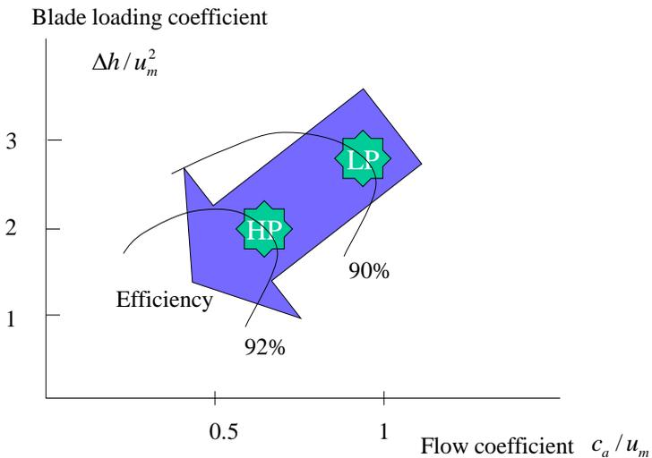
**Fig. 13.16 Turbine efficiency versus flow and blade loading coefficients**
