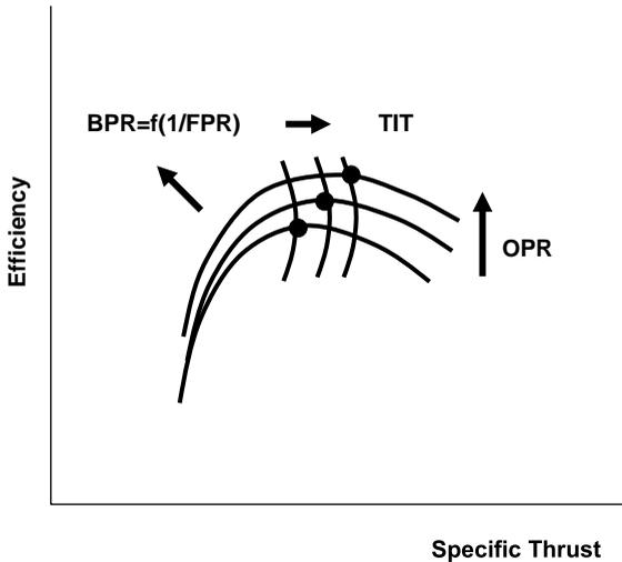
**Fig. 12.9** Typical relationships between the main parameters
