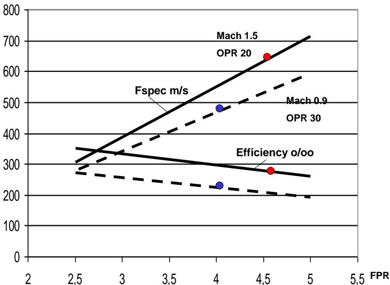
**Fig. 16.11 Specific thrust and efficiency versus FPR for different Mach numbers**
