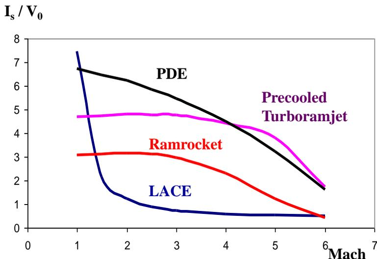
**Fig. 21.9** Specific impulse of engines for speeds below Mach 6
