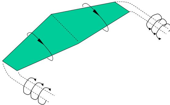
**Fig. 7.4 Trailing vortices from wingtips give rise to induced drag**
