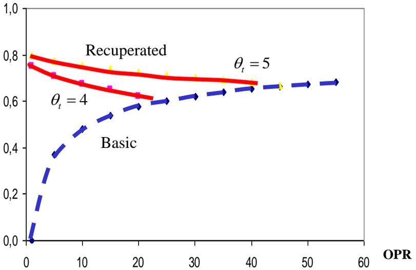
**Fig. 14.3 Variation of recuperated thermal efficiency with pressure**
