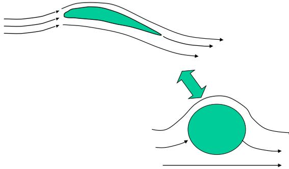
**Fig.7.2 Joukowski transformed the flow around an airfoil to that around a cylinder**
