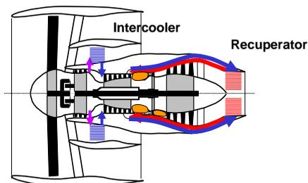
**Fig. 14.8 Effect of combined recuperators and intercoolers**
