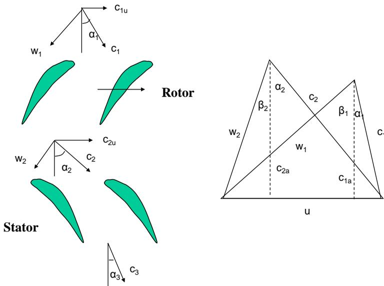
**Fig. 13.4 Cascade flow and velocity triangles**
