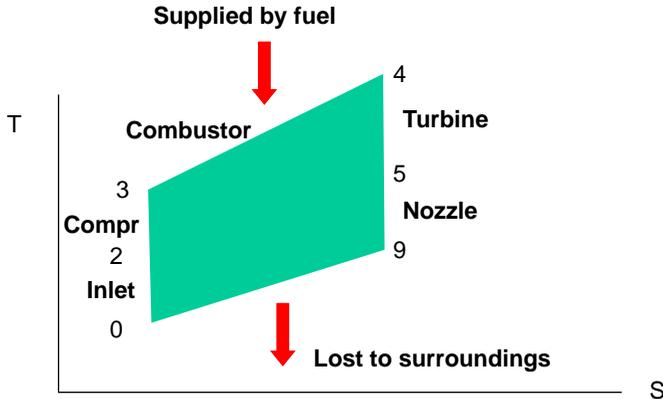
**Fig. 8.8 The jet engine follows the Brayton cycle**
