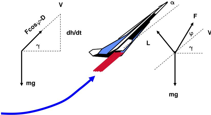
**Fig. 15.4 Forces on a climbing aircraft**
