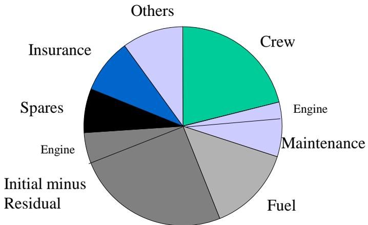
**Fig. 10.3 The typical distribution of costs for an aircraft**
