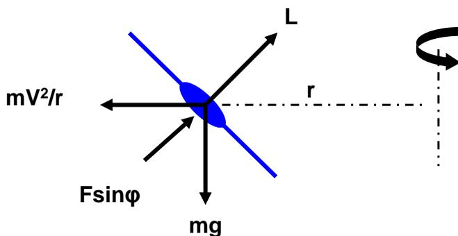
**Fig. 15.7 Forces on a turning aircraft**
