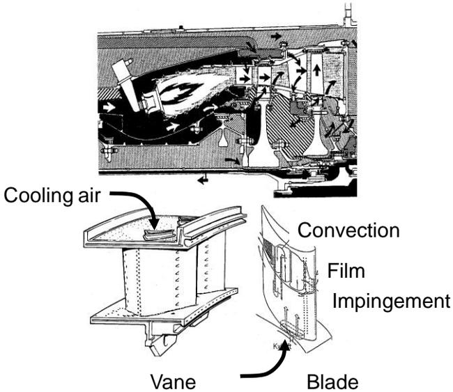
**Fig. 13.14 Turbine with cooling flows**
