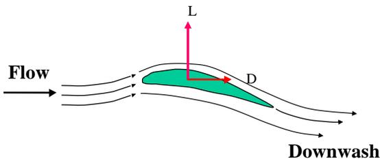
**Fig. 5.7 The lifting wing**
