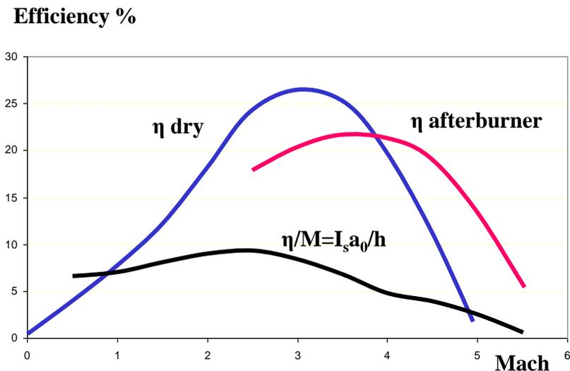
**Fig. 21.6 The efficiency of a ramrocket with and without afterburner.**
