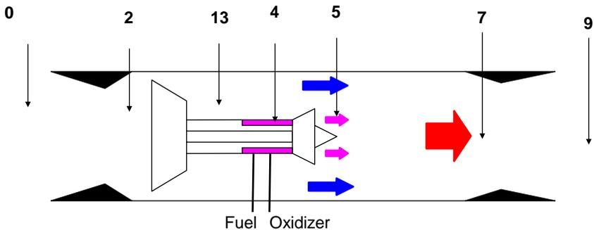
**Fig. 21.2** In the Turboramrocket, the rocket exhaust gases are used to drive the turbine for the fan
