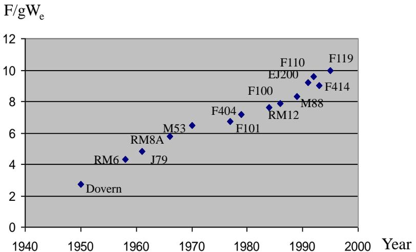
**Fig. 16.2 How the thrust-to weight ratio of engines has increased with time**
