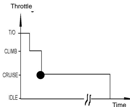
**Fig. 11.12 The engine is designed for beginning of cruise**
