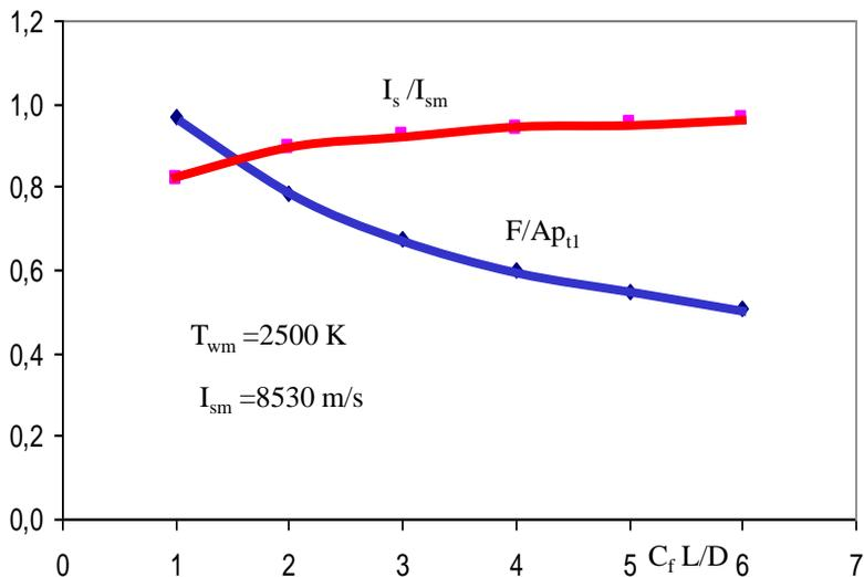
**Fig. 23.5 Specific impulse and thrust for a nuclear engine**
