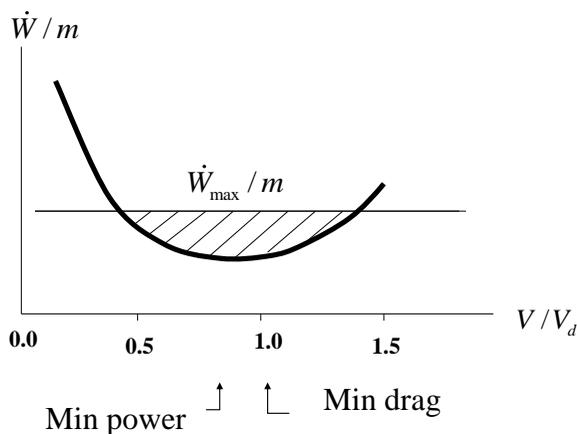
**Fig. 4.4 The flight power curve**
