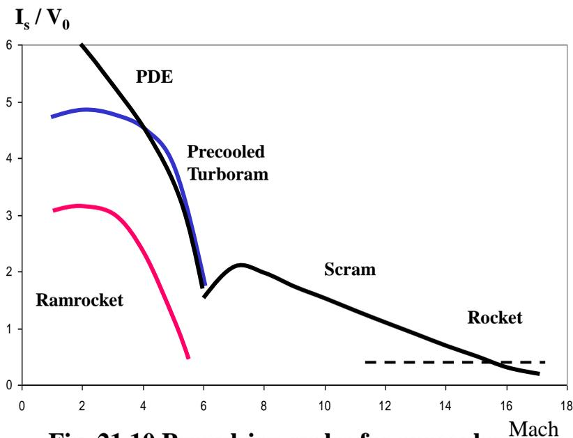
**Fig. 21.10 Propulsion cycles for spaceplanes**
