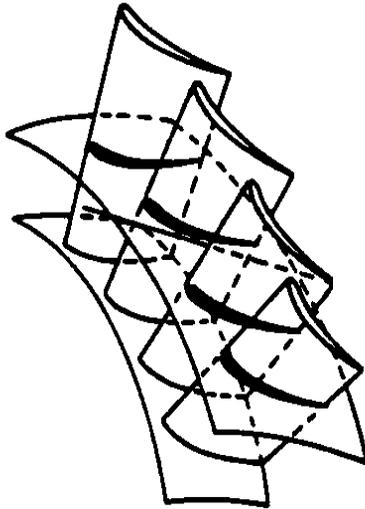
**Fig. 13.3 Blade stream surfaces**
