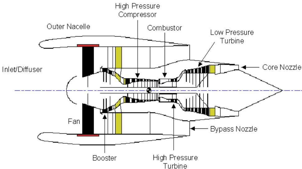
**Fig. 9.7 The components of the bypass engine**
