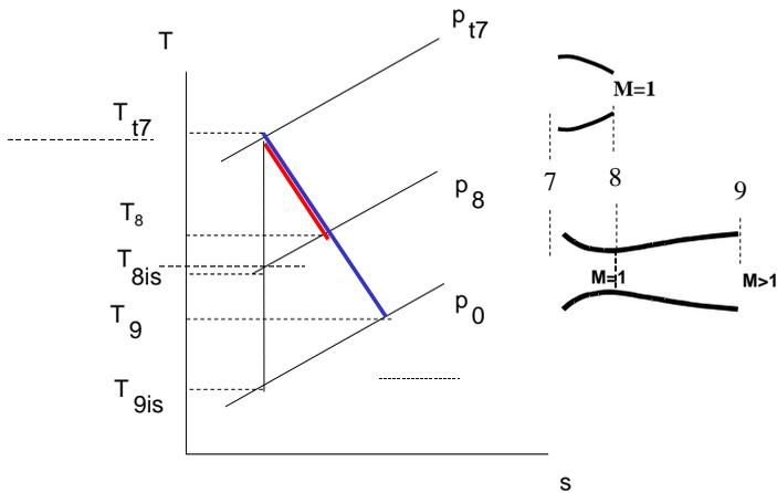
**Fig. 16.7** Expansion in a **convergent-divergent** and in a **convergent** nozzle
