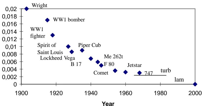
**Fig. 11.9 The aircraft parasite drag is approaching that of a turbulent flat plate**
