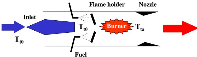
Fig. 19.1 The principle of a ramjet
