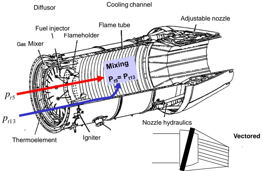
**Fig. 16.6** The afterburner and nozzle distinguishes a military engine
