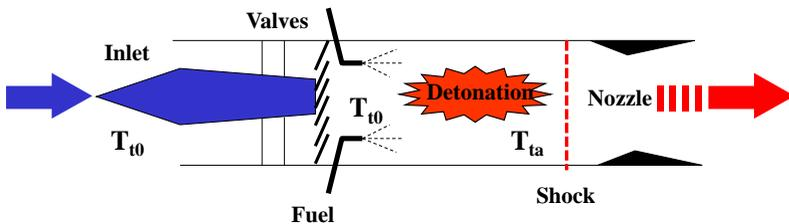
**Fig. 19.2 The principle of a Pulse Detonation Engine**
