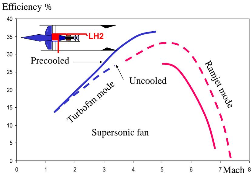
**Fig. 18.7 Increased efficiency with precooling**
