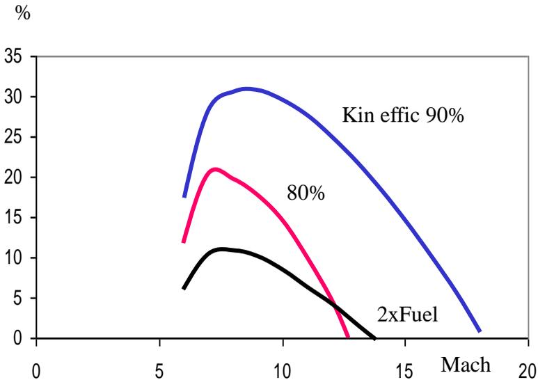
**Fig. 19.7 The efficiency of a Scramjet**
