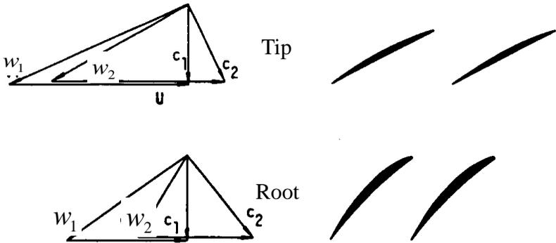
**Fig. 13.9 Blade shapes at tip and at root.**
