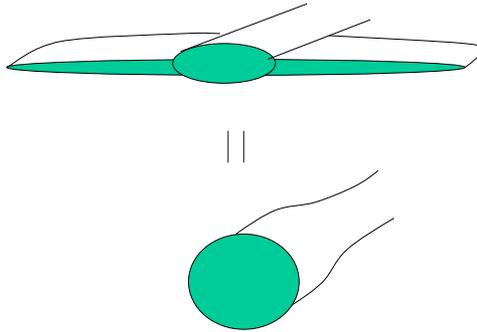
**Fig. 8.10 The area rule for the design of supersonic aircraft**
