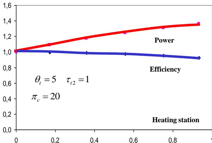
**Fig. 14.6 Power and efficiency with reheating**
