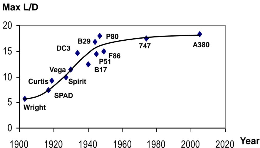
**Fig. 11.8 Stagnating Lift/Drag ratio**
