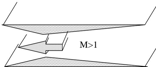
**Fig. 19.6 The supersonic ramjet (Scramjet)**
