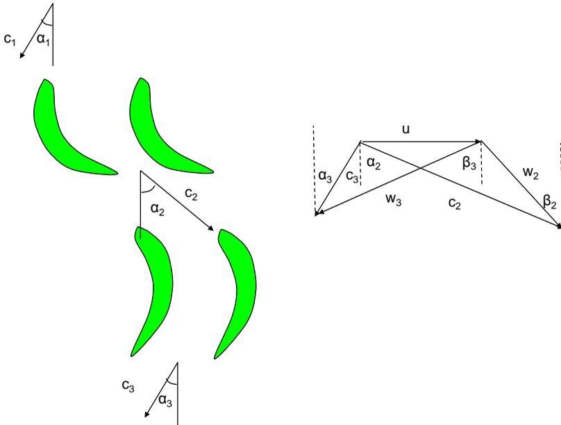
**Fig. 13.17 Turbine cascade with velocity triangles**
