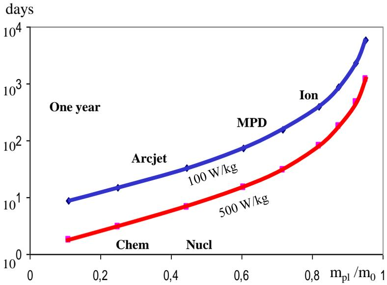
**Fig. 23.8 Operating time with optimum payload**
