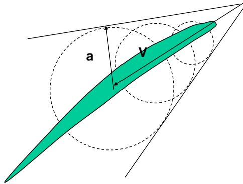
**Fig. 7.8 Shocks at a blade tip at supersonic speed**
