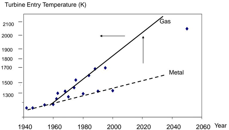
**Fig. 12.10** The increase of the Turbine Entry Temperature
