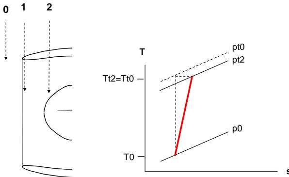
**Fig. 12.2 The inlet has a small pressure loss**
