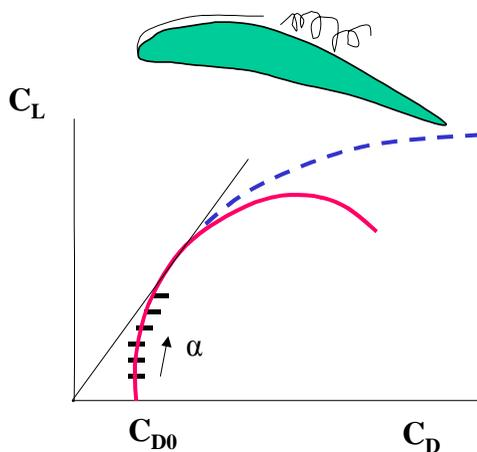
**Fig. 6.4** The maximum L/D is at the tangent to the drag polar
