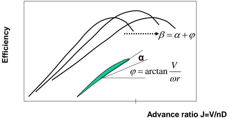
**Fig. 7.7 The propeller has maximum efficiency for a certain advance ratio**
