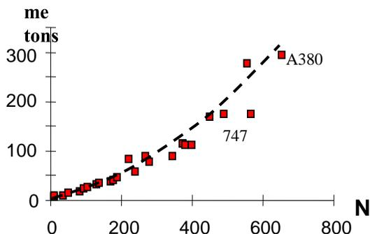
**Fig. 11.2 The empty weight of aircraft vs the number of passengers**
