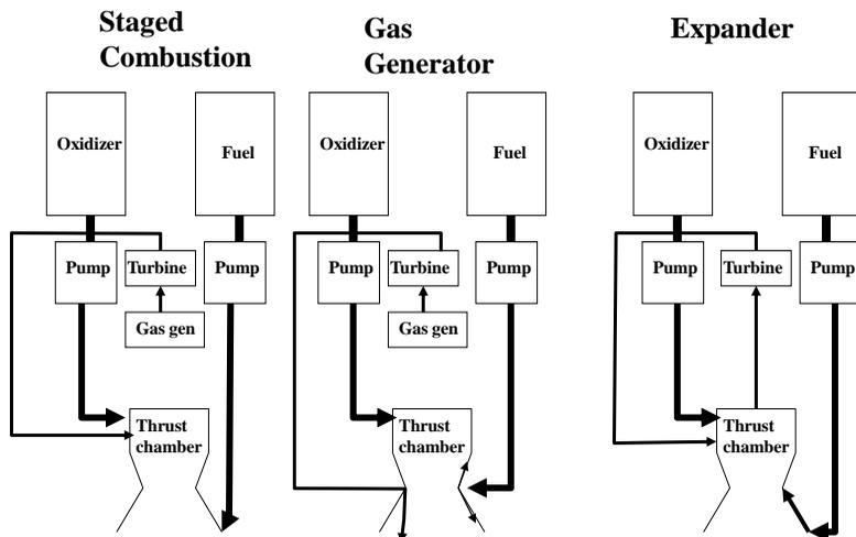
**Fig. 20.3 Pump-fed liquid rocket engine cycles**
