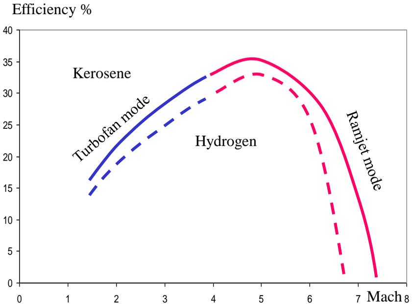
**Fig. 18.6 Decreased efficiency with hydrogen**
