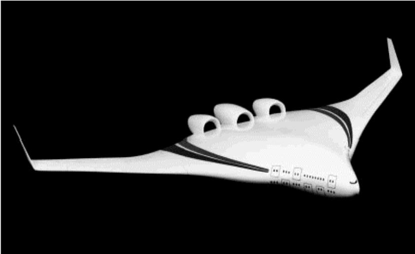
**Fig. 11.10 The blended body aircraft**
