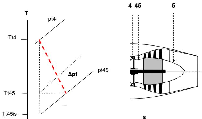
**Fig. 12.7 Pressure and temperature losses in the turbine**
