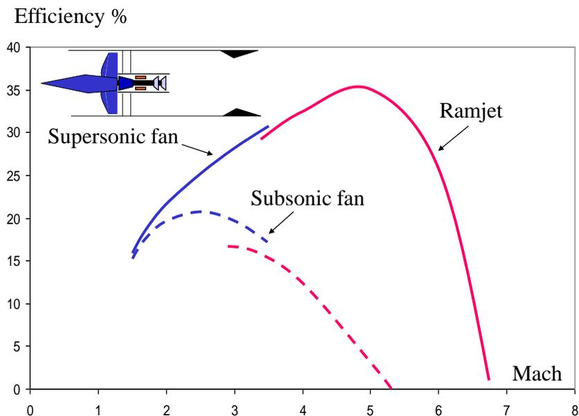
**Fig. 18.5 Increased efficiency with a supersonic fan**
