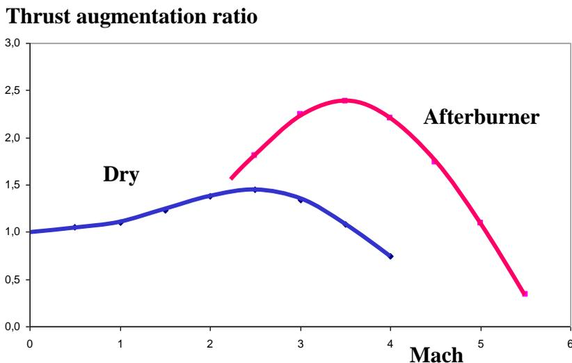
**Fig. 21.5** The ratio between the ramrocket thrust and the rocket thrust.
