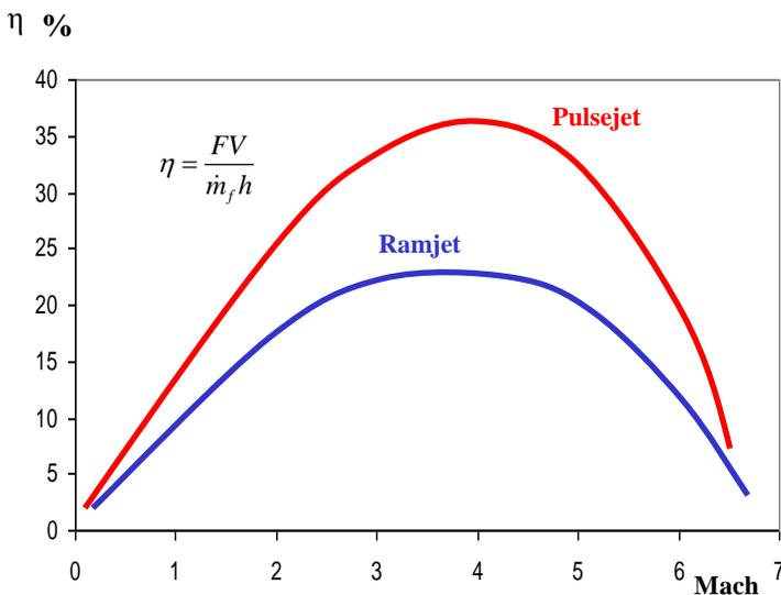
**Fig. 19.3** The PDE is more efficient than the ramjet
