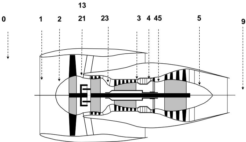
**Fig. 12.1 Section numbering of a bypass engine**
