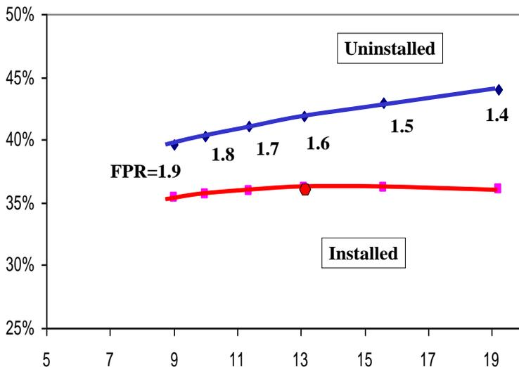
**Fig. 12.11 The efficiency has a maximum for a certain Bypass Ratio (BPR)**
