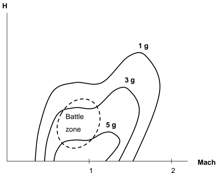
**Fig. 15.8 Sustained turn flight envelopes for different load factors**
