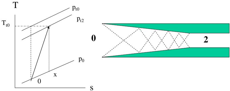
**Fig. 18.3 Pressure loss in inlets**
