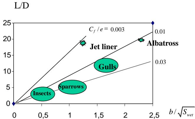
**Fig. 5.5 The Lift-to-Drag ratio of birds**
