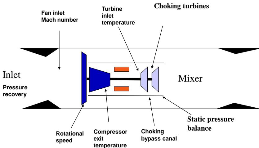
**Fig. 18.1 Limitations in the operation of the jet engine**
