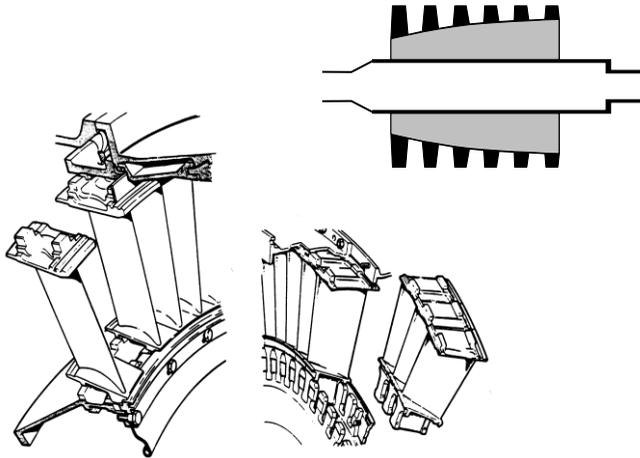
**Fig. 13.2 Axial flow compressor blades and vanes**
