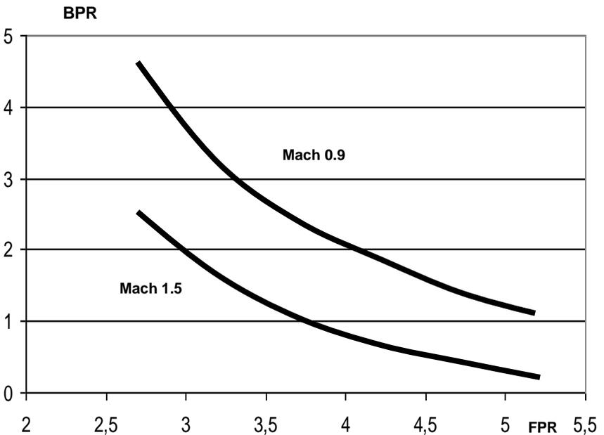
**Fig. 16.12** The bypass ratio decreases with fan pressure ratio
