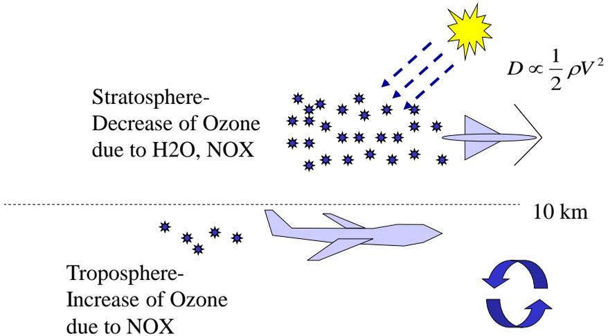
**Fig. 10.6 The influence on ultraviolet radiation depends on flight altitude**
