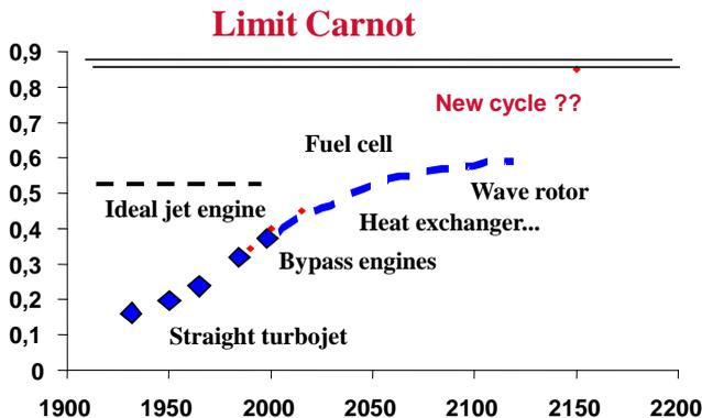
**Fig. 14.10 Limits of the turbojet**
