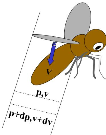
**Fig. 3.4 The reaction force is balanced by a pressure force below the wings.**
