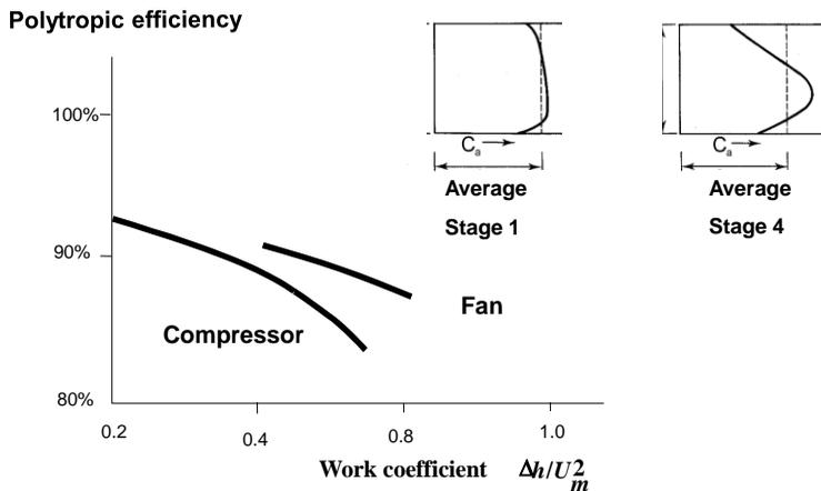
**Fig. 13.10 The efficiency decreases as the work coefficient increases**
