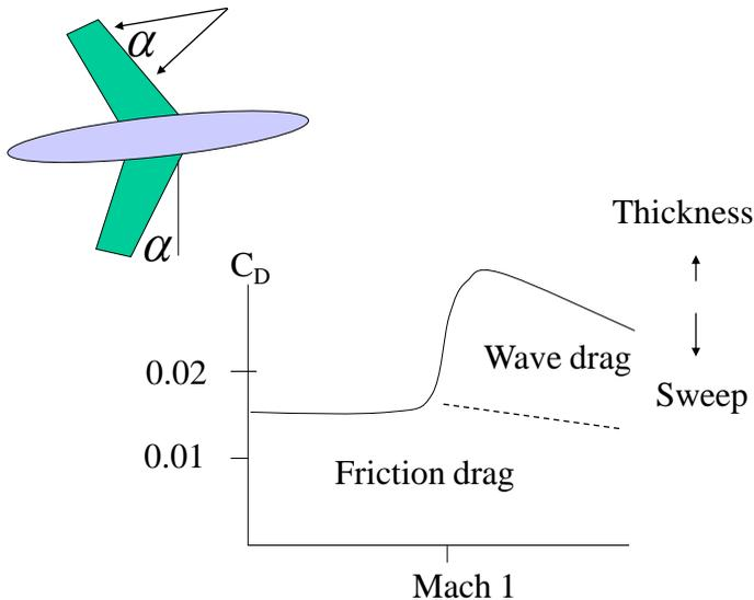
**Fig. 8.9** The sonic barrier is seen as a large increase in drag
