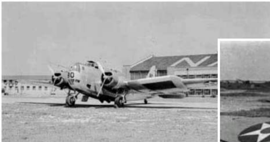
LFC glove (slot type) at Douglas B18 (NACA, Langley Research Center 1941)
