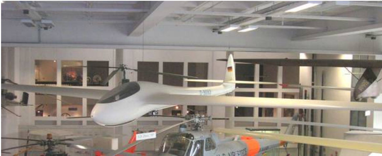
First all fiberglass -composite based composite fs 24 Phönix (1957). The choice of material offered to gain substantial benefit from natural laminarity (max. total L/D 1:40)
