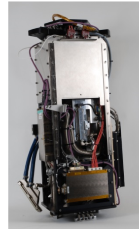
isothermal solidification exp. with furnace using X-ray as diagnostic tool
