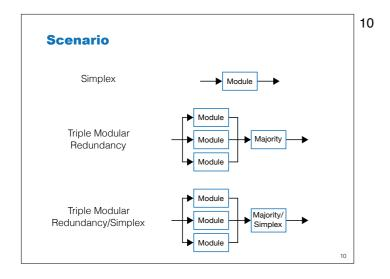
To show how it applies to fault-tolerant systems context, lets consider three kinds of fault tolerance schemes: simplex, TMR and TMR/Simplex. On Simplex, we have no fault-tolerance at all. It is simple and cheap on design resources. On TMR we have replicated modules and the results of the module are taken by a majority voter. For the TMR/Simplex, when a module fails, we put a good module aside.
