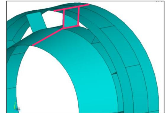
Find the *stiffest & lightest TRS geometry* for a certain turbine by *varying the geometrical position of TRS vanes*
