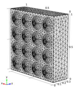
freq(1)=200 Hz Surface: Total acoustic pressure field (Pa) 0 0.1 0.2 0.30
