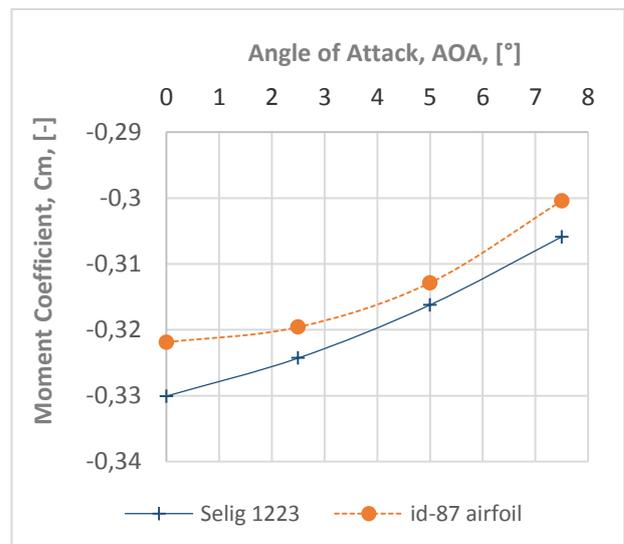
**Figure 8: Moment Coefficient vs AOA**
