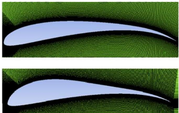
**Figure 3: Different Airfoils with Similar Meshes.**
