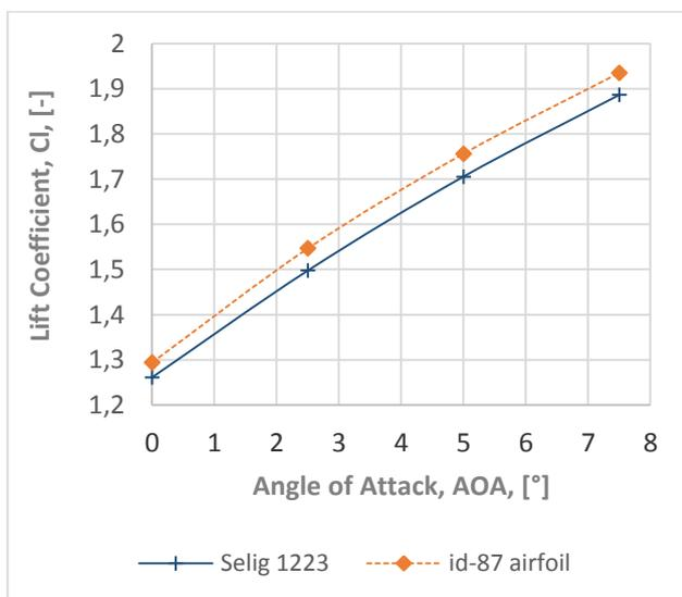
**Figure 7: Lift Coefficient vs AOA**
