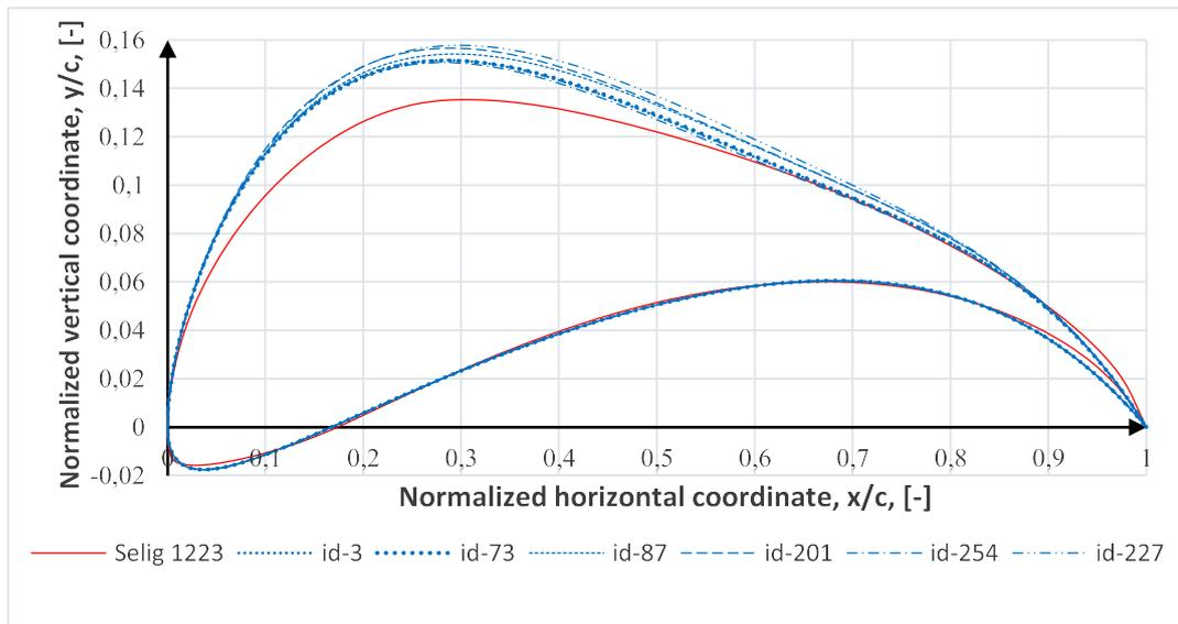
**Figure 6: Comparison between the Obtained Solutions and the Original Selig 1223**
