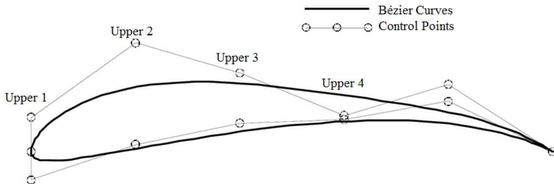
**Figure 2: The Selig 1223 High Lift Airfoil and its Control Points**
