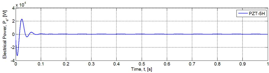
**Figure 8: Electrical Power of PZT-5H.**
