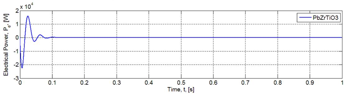
**Figure 6: Electrical Power of PbZrTiO3.**
