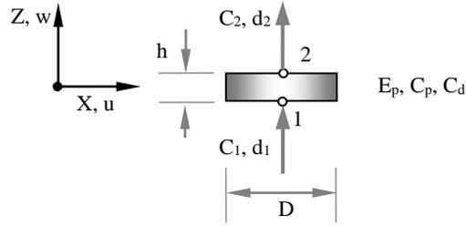
**Figure 2: The uniaxial finite element of a piezoelectric crystal.**
