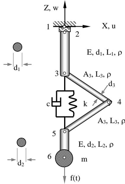
**Figure 1: Landing gear model.**
