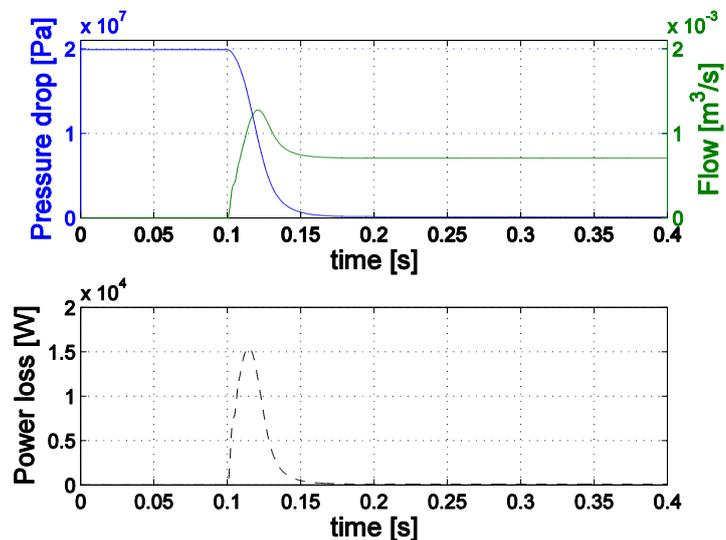
Figure 1. Power loss during a valve opening
