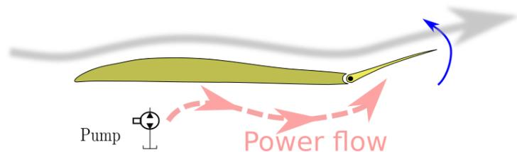
Figure 2. Power from the pump to the control surface
