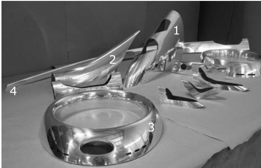
Superplastically components formed in SP5083, 1. wing tip light housings 2. strakelets, 3. engine intake lipskins and 4. winglet (SUPERFORM®)
