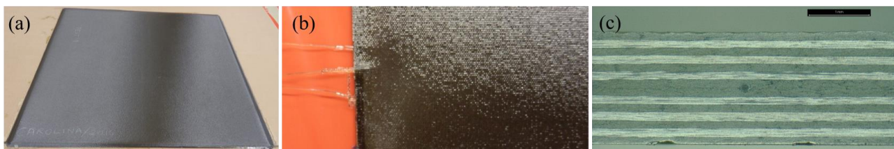
Figure 2. (a) Composite board with embedded optical fibers; (b) detail of the embedded fibers insertion point; (c) transversal cut view of a composite sample with embedded fiber in its 90^\circ/90^\circ mid layer.
