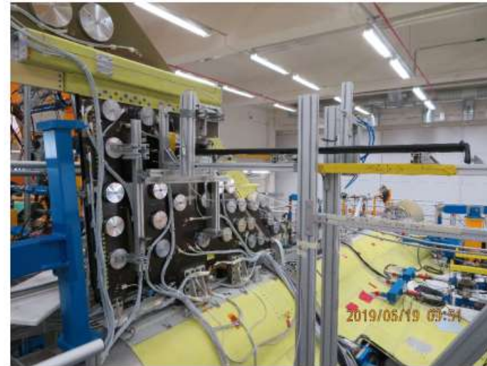
Figure 4 - Test setup for impact tests on the fin.
