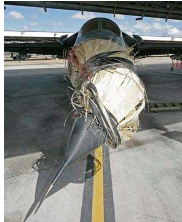
F-111 A8-112, collision with a pelican, Amberley 11th April 2008 Photo: Darren Crick, RAAF
