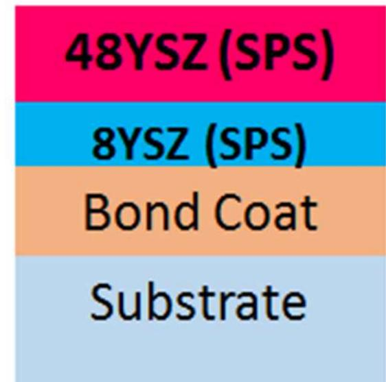
Different TBCs sprayed by suspension plasma spray process
