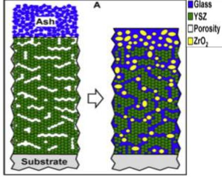
Schematic of CMAS degradation, Padture et al.
