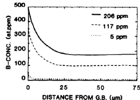
Fig. 6. Simulated segregation profiles in austenite with 206, 17 or 5 at. ppm boron. The starting temperature was 1250  $^{\circ}\text{C}$ , the cooling rate 100  $^{\circ}\text{C/s}$  and the calculations were performed using Set 1 (Table 1) parameter values for a grain size of 150  $\mu\text{m}$ .
