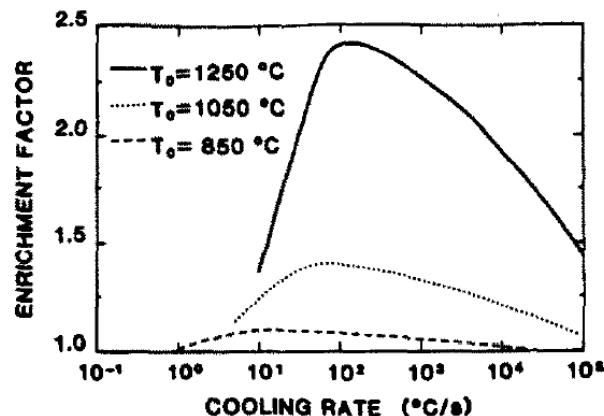
Fig. 8. Calculated enrichment factors i.e. the boron concentration within 375 nm of the boundary divided by the bulk concentration as a function of cooling rate for starting temperatures 1250, 1050, and 850  $^{\circ}\text{C}$ . Austenite with 206 at. ppm boron, grain size 150  $\mu\text{m}$  and using Set 1 (Table 1) parameter values.
