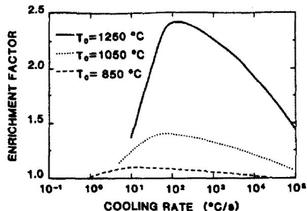
Fig. 8. Calculated enrichment factors i.e. the boron concentration within 375 nm of the boundary divided by the bulk concentration as a function of cooling rate for starting temperatures 1250, 1050, and 850°C. Austenite with 206 at. ppm boron, grain size 150  $\mu\text{m}$  and using Set 1 (Table 1) parameter values.
