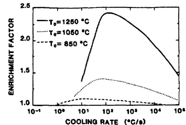
Fig. 8. Calculated enrichment factors i.e. the boron concentration within 375 nm of the boundary divided by the bulk concentration as a function of cooling rate for starting temperatures 1250, 1050, and 850 $^{\circ}\text{C}$ . Austenite with 206 at. ppm boron, grain size 150  $\mu\text{m}$  and using Set 1 (Table 1) parameter values.
