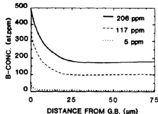
Fig. 6. Simulated segregation profiles in austenite with 206, 17 or 5 at. ppm boron. The starting temperature was 1250°C, the cooling rate 100°C/s and the calculations were performed using Set 1 (Table 1) parameter values for a grain size of 150  $\mu\text{m}$ .
