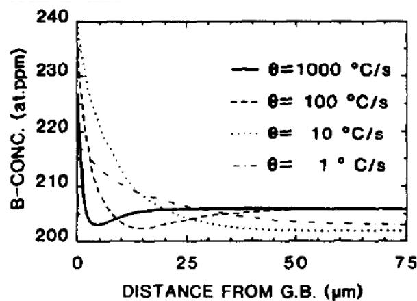
Fig. 3. Simulated segregation profiles in austenite with 206 at. ppm boron after cooling at 1000, 100, 10 and 1  $^{\circ}\text{C/s}$ . The starting temperature was 1250  $^{\circ}\text{C}$ , the grain size 150  $\mu\text{m}$  and Set 2 (Table 1) parameter values were used.
