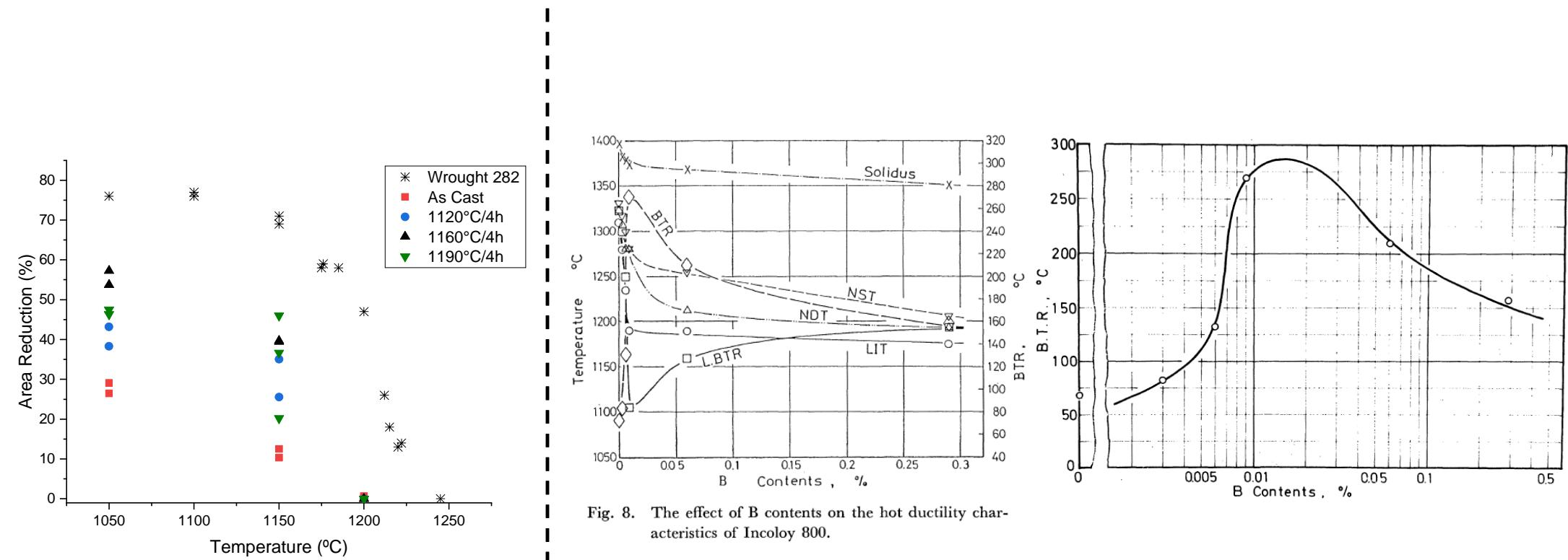
Fig. 8. The effect of B contents on the hot ductility characteristics of Incoloy 800.
