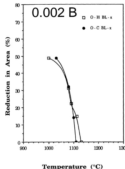
Fig. 56: Percent Reduction in Area Versus Test Temperature From On-Heating and On-Cooling Hot-Ductility Tests of Cast Controlled Boron Heat BL.
