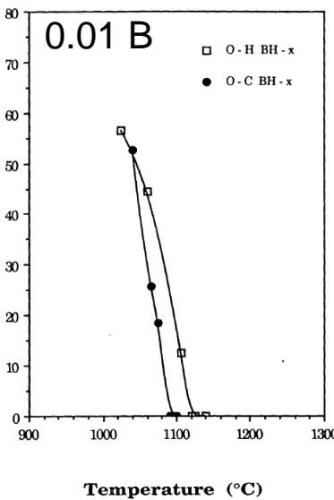
Percent Reduction in Area Versus Test Temperature From On-Heating and On-Cooling Hot-Ductility Tests of Cast Controlled Boron Heat BH.
