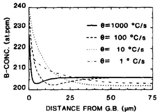
Fig. 3. Simulated segregation profiles in austenite with 206 at. ppm boron after cooling at 1000, 100, 10 and 1°C/s. The starting temperature was 1250°C, the grain size 150  $\mu\text{m}$  and Set 2 (Table 1) parameter values were used.
