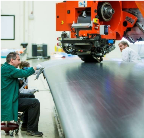
Hand lay-up vs. automated lay-up
