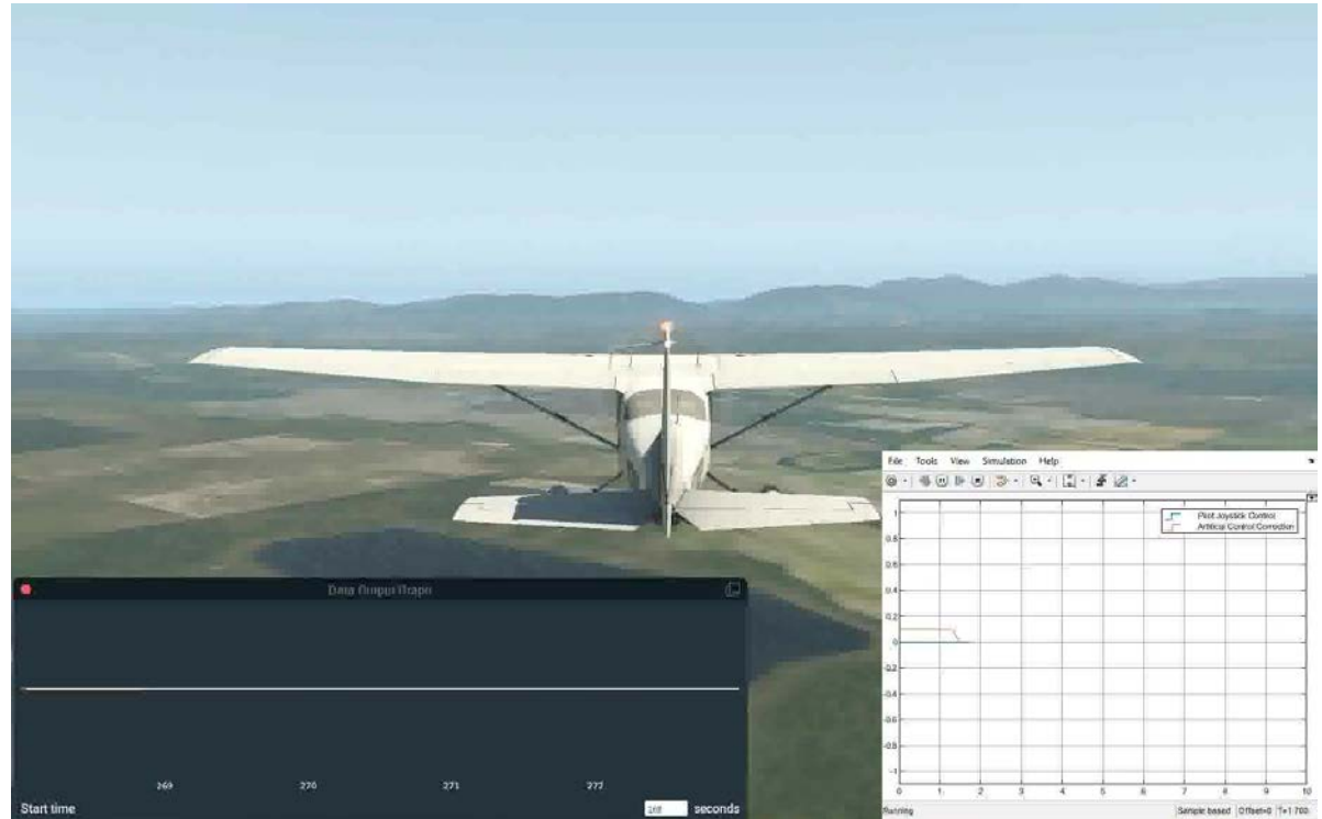
Aileron control signal from the pilot and the Simulink roll control model
