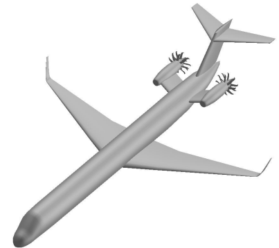
Single-aisle airplane w/rear-mounted open rotors
