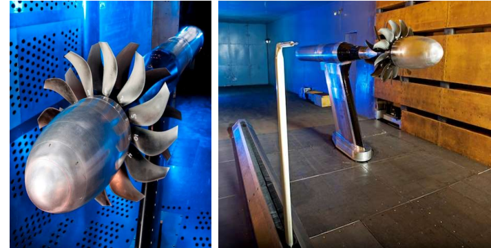
Open Rotor Propulsion Rig installed in GRC's 8x6 (left) and 9x15 (right) Wind Tunnels
