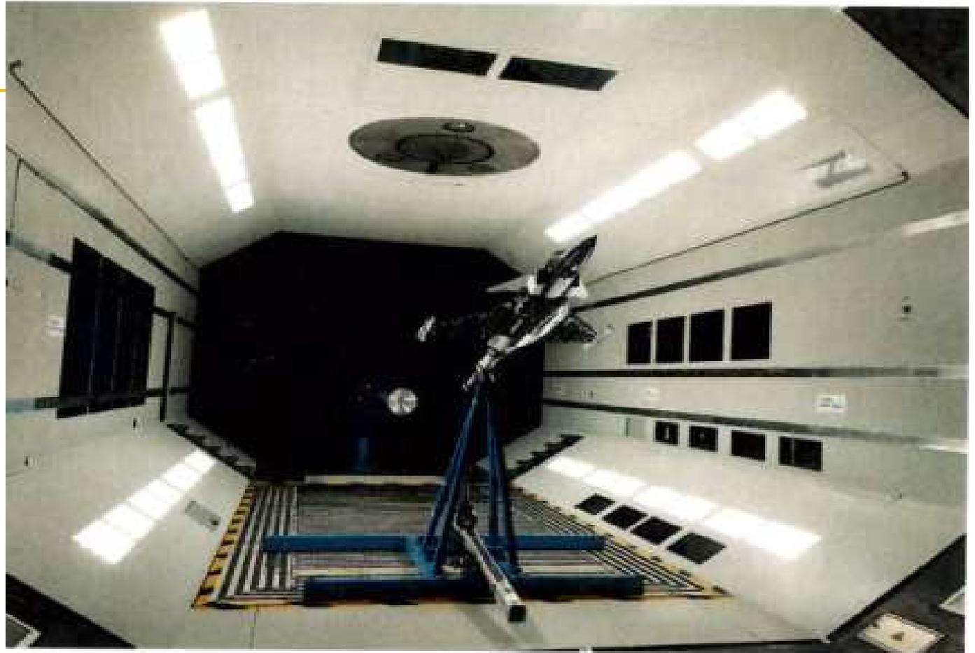
**Figure 1:** The test-setup used in the wind tunnel in Emmem.
