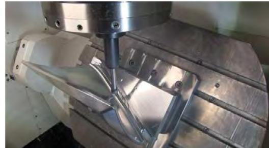
Figure 14 Multi axis machine tool configuration, Courtesy of Precise Tool and Manufacturing; Rochester, NY 14624
