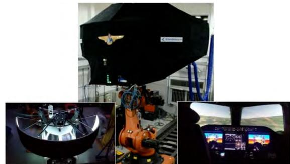
Figure 1: SIVOR – robotic flight simulator.
