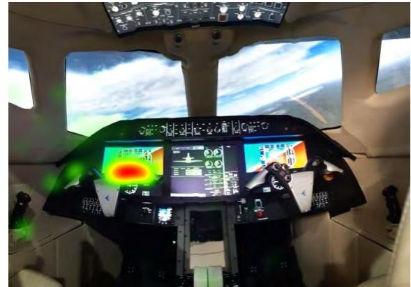
Figure 5: heat map of the pilot's vision focused area during an attempt of compensating a system failure.
