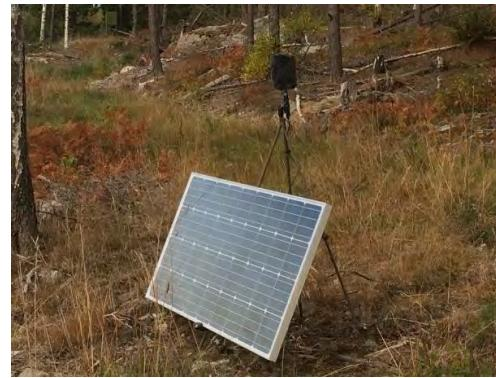
*Figure 1: Photo of the acoustic measurement station. Depicted is the solar cell and the microphone with fitted windsreen*
