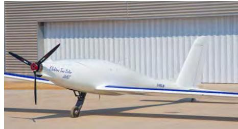
Figure 1: Autonomous solar-powered aircraft: Elektra 2.
