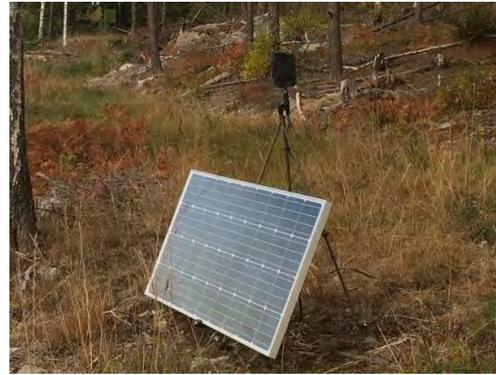
*Figure 1: Photo of the acoustic measurement station. Depicted is the solar cell and the microphone with fitted windscreen*
