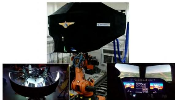
Figure 1: SIVOR – robotic flight simulator.
