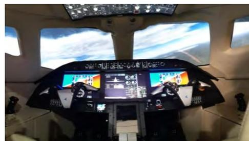
Figure 2: SIVOR's flexible cockpit with main flight deck, yoke and stick inceptors and virtual overhead panel.
