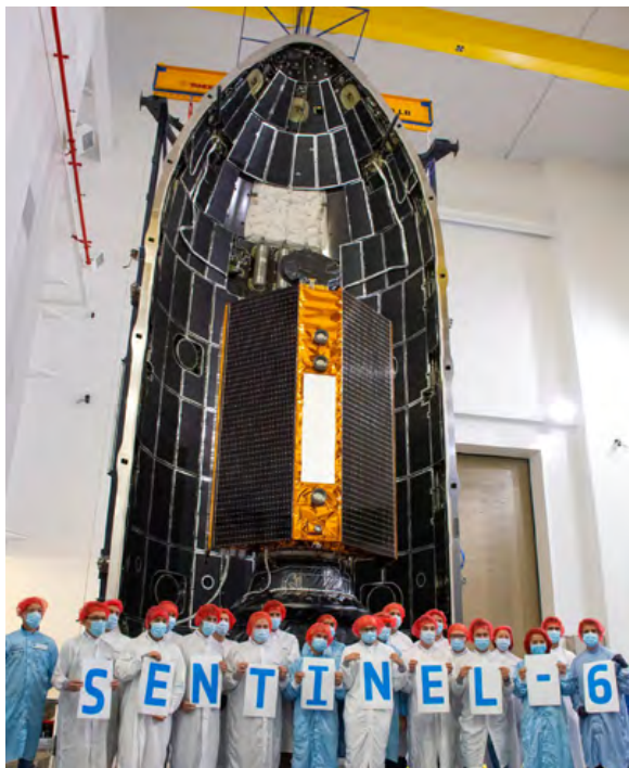
Inside SpaceX's Payload Processing Facility at Vandenberg US Air Force Base (CAL), the US-European Sentinel-6 Michael Freilich is being encapsulated in the SpaceX Falcon 9 payload fairing, 3 November 2020. © Credit NASA
