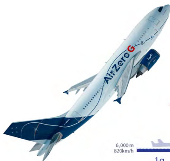
Figure 1 - The whole parabolic flight maneuver comprises three phases: 20-second pull-up – 22-second ballistic phase – 20-second pull-out.
