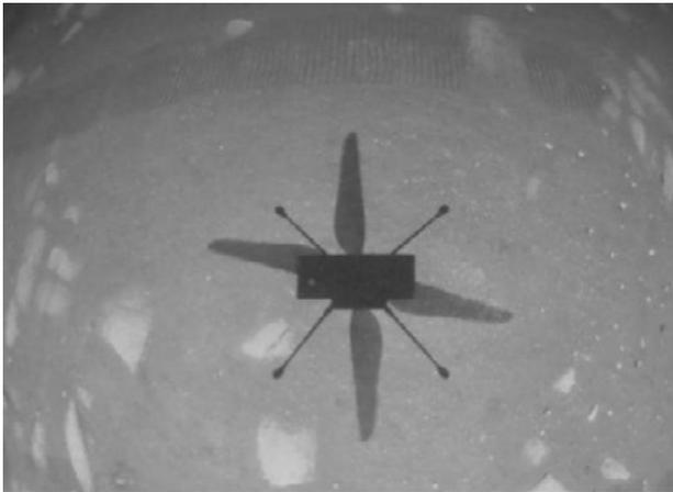
*NASA's Ingenuity Mars Helicopter captured this shot as it hovered over the Martian surface on 19 April 2021, during the first instance of powered, controlled flight on another planet. It used its navigation camera, which automatically tracks the ground during flight. Credits: NASA/JPL-Caltech*
