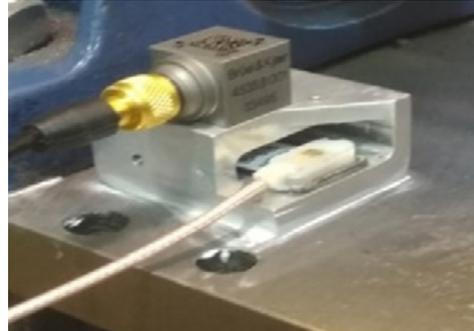
*Sensors are packaged into a light weight assembly with a small footprint*
