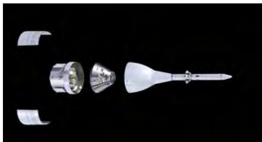
Figure 8 Orion is made of three main sections. From the left: (1) The service module, from the European Space Agency, fuels and propels the spacecraft. (2) The crew module is the habitat for up to four astronauts. (3) The Launch Abort System detaches and flies away after Orion reaches orbit. © NASA
