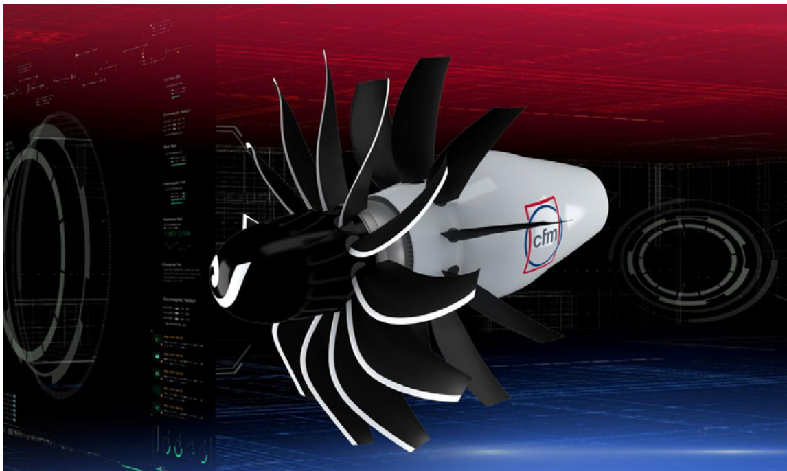
Figure 1 : GE and Safran are evaluating several promising architectures as part of their technology maturation plan. The most ambitious, the one that will yield the greatest benefit – is open fan architecture. © Safran Group.
