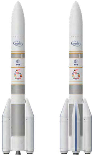
Illustration of the two Ariane 6 variants planned, A62 (left) and A64 (right)
