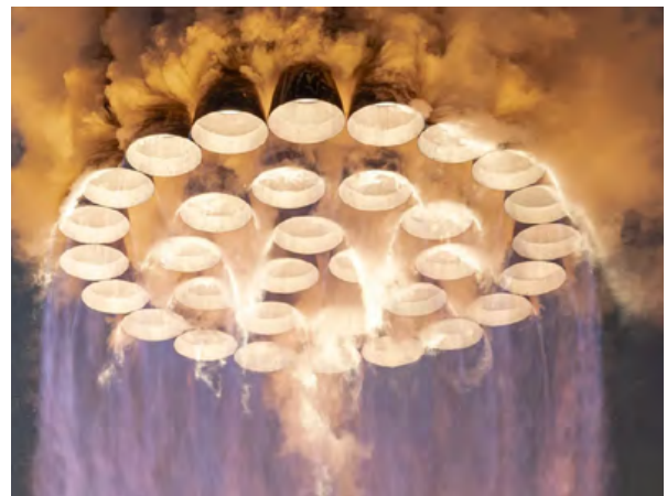
Illustration 2 SpaceX's giant Starship rocket launched on its second-ever test flight on Nov. 18, 2023, igniting all 33 of its first-stage Raptor engines in unison for lift-off. (Image credit: SpaceX)
