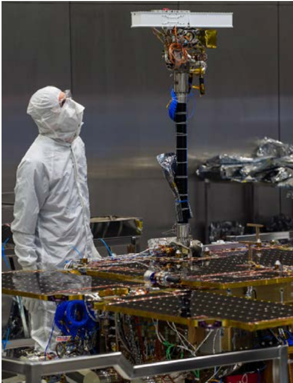
The ExoMars (Rosalind Franklin) Rover being checked during integration activities inside the Bio CleanFacility at Airbus Stevenage (UK). Credit: Airbus
