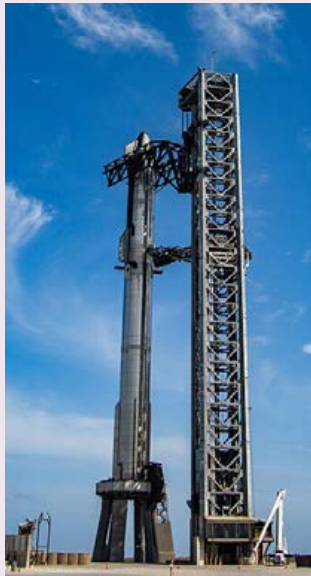
Starship prototype in launch configuration: Starship spacecraft sits on top of Super Heavy.
