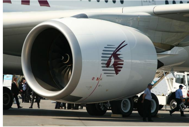
Rolls-Royce Trent XWB (A350) BPR = 9.6 Specific Fuel Consumption: 13.5 \text{ g/kN}\cdot\text{s}
