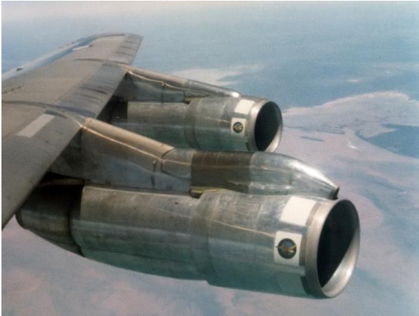
Pratt & Whitney JT3D (B707) BPR = 1.42 Specific Fuel Consumption: 22 \text{ g/kN}\cdot\text{s}
