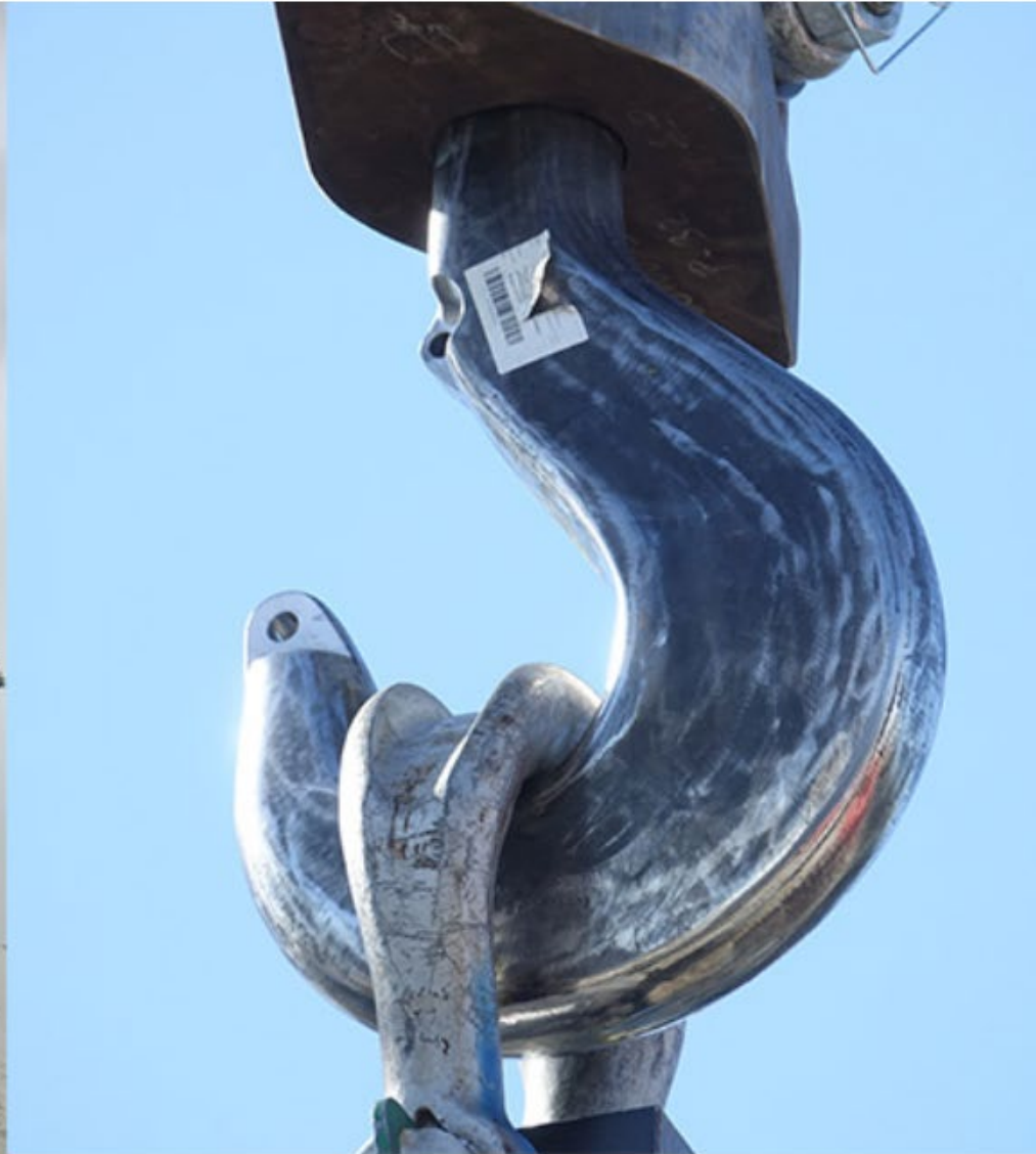
[A 3D-printed metal hook [Image credit: Huisman Equipment]]
