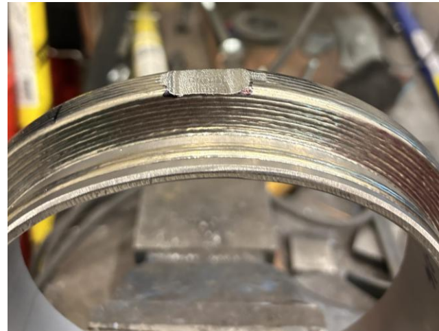
Manual groove preparation
